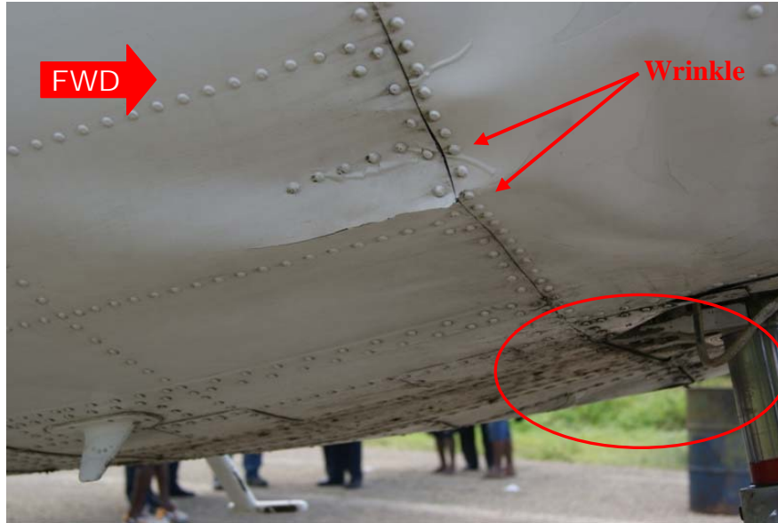
Figure 2. PK-NUH Station 60 (Lower Fuselage) Section
