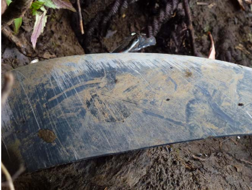
Figure 3: Scratch marks found on the propeller leading edge.
