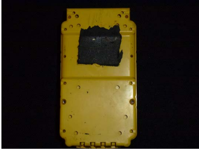
Figure 4: The ELT installation used double tape instead of fastener
