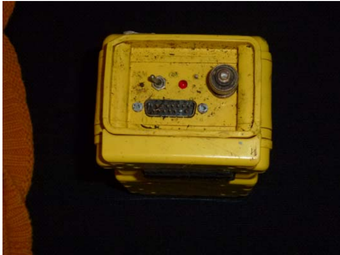
Figure 5: The antenna detached from the ELT unit.
