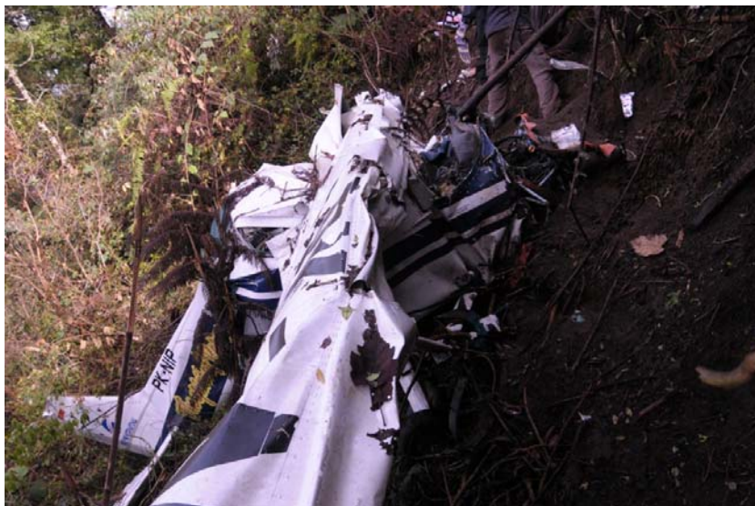
Figure 2: Damage on the wing leading edge and forward section.
