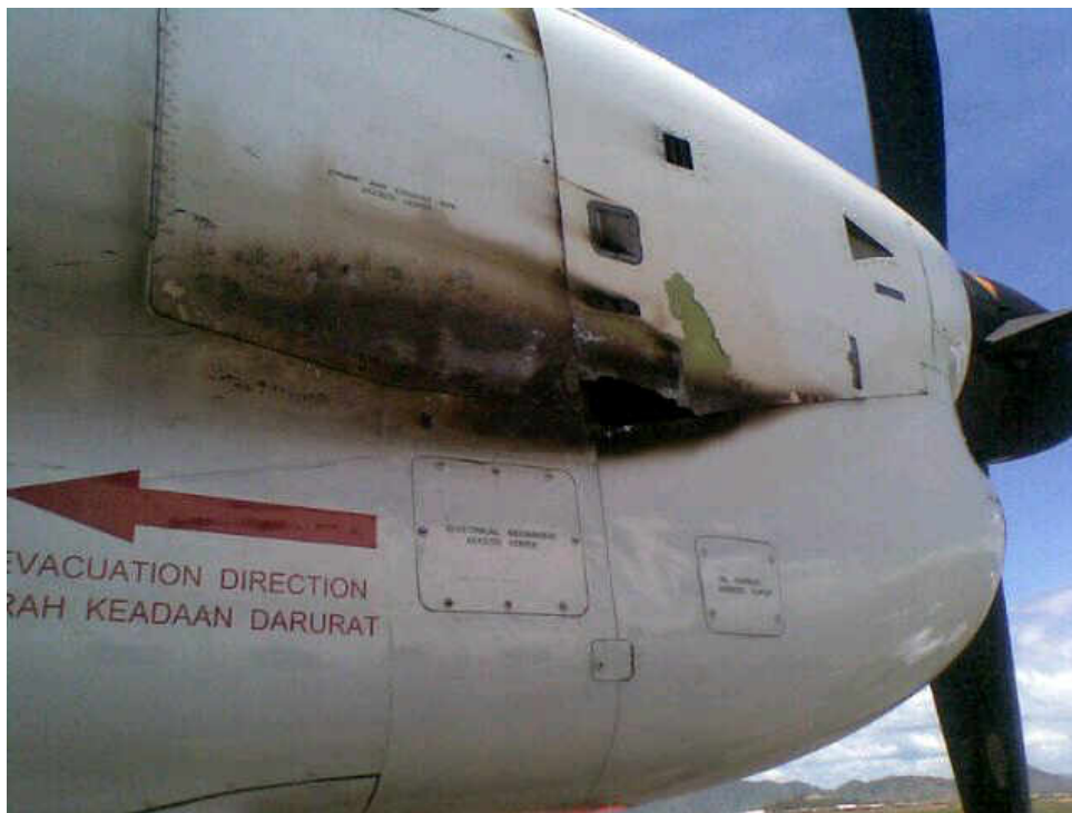
Figure 1: The left engine cowling was damaged
