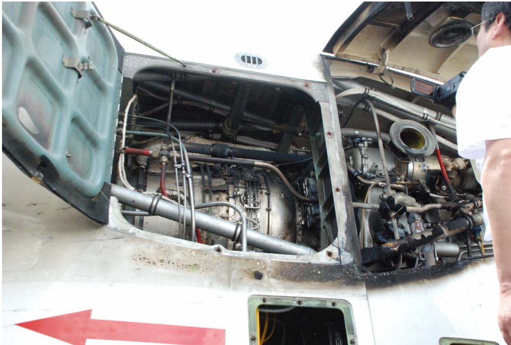
Figure 10: Signature of fire in front of bulkhead frame
