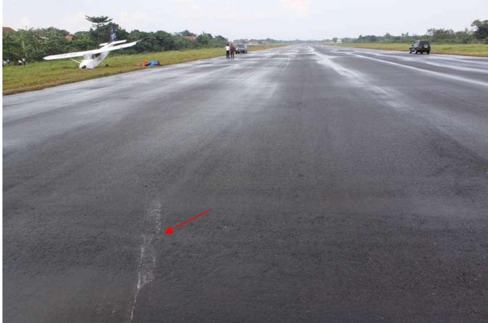
Figure 3: The left wing tip paint mark
