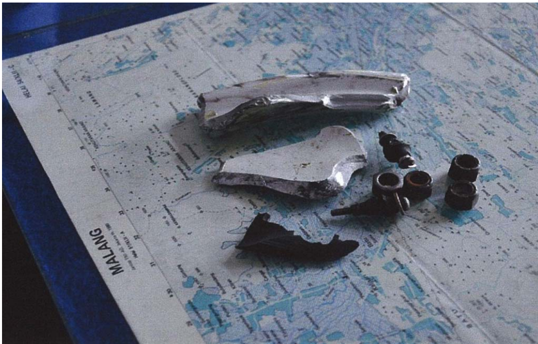
Figure 8: The broken parts of nose wheel hub
