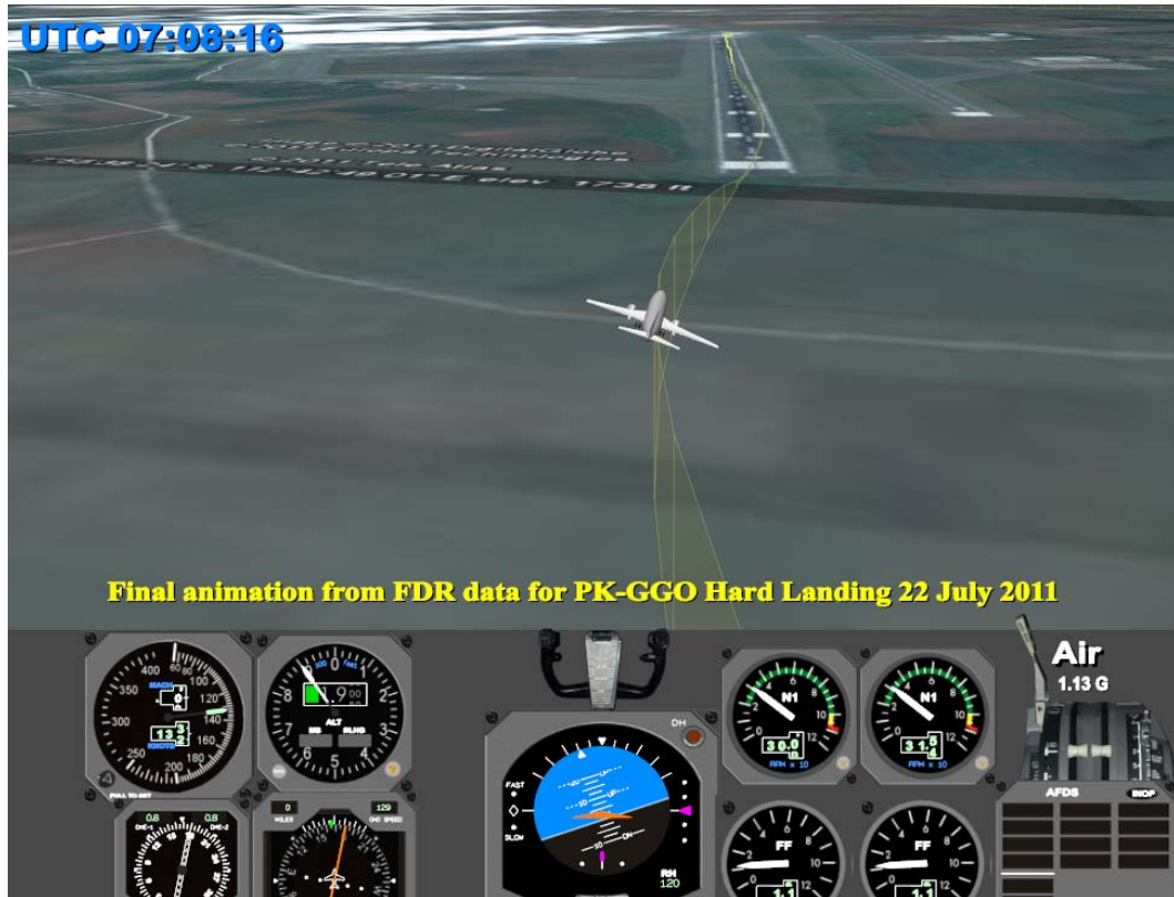
Figure 1: The flight profile from approximately 300 feet AGL based on FDR animation
