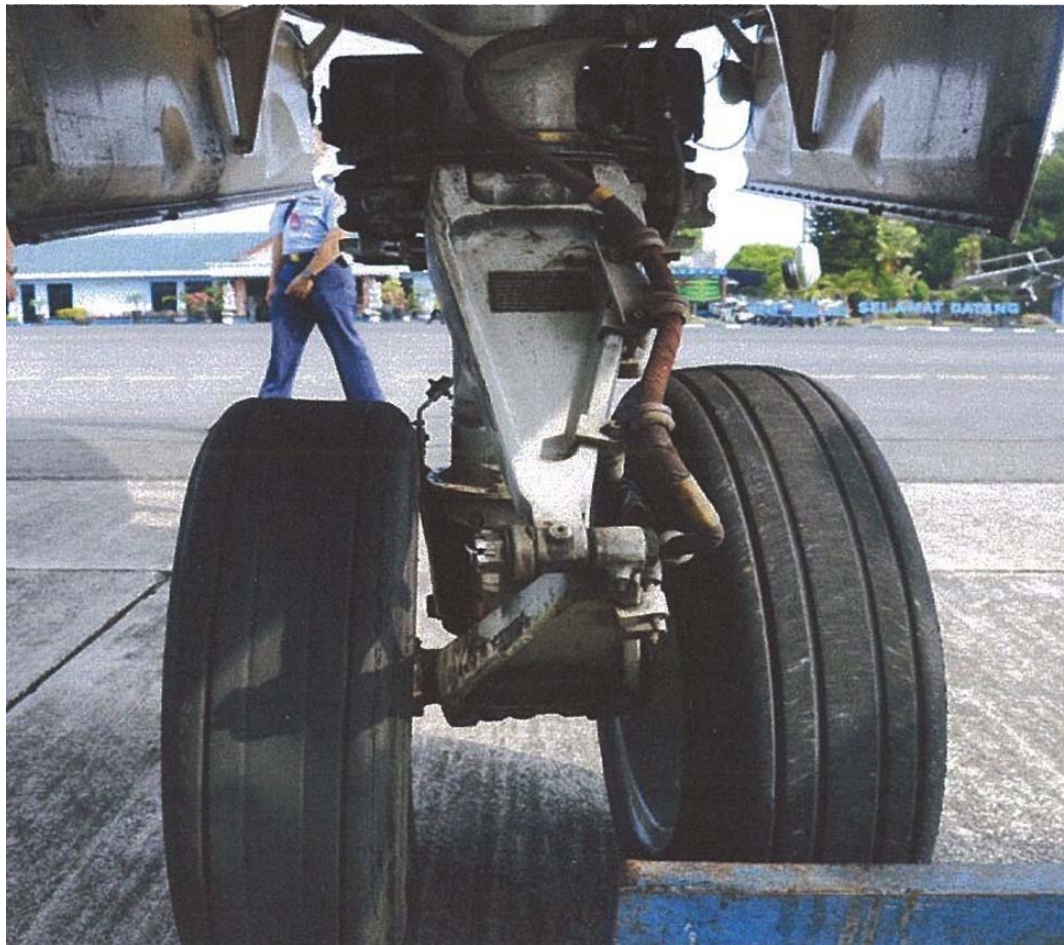
Figure4: The damage on the nose landing gear
