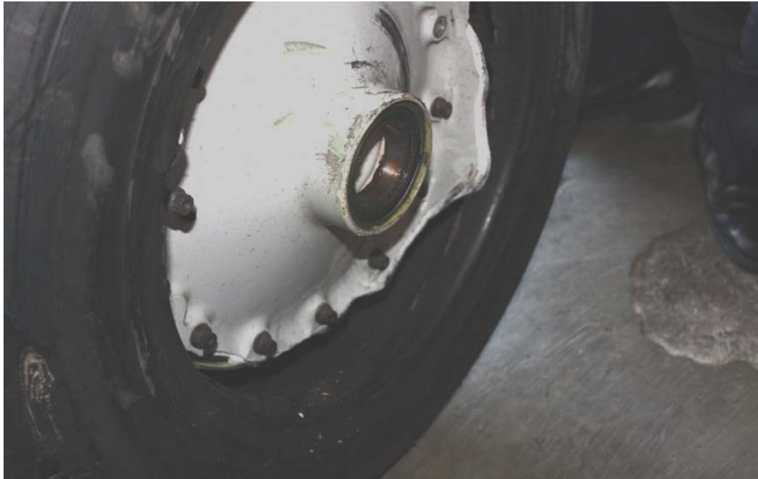
Figure 9: The damage on the nose wheel hub
