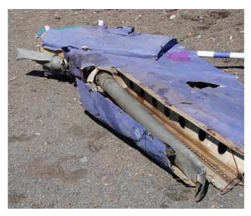
Figure 8: Twisted tail rotor shaft
