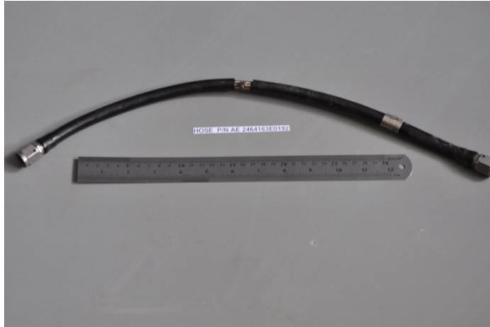
Figure 7: The hose shows damage in the middle
