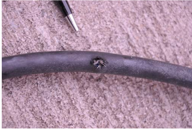
Figure 1: Hydraulic Hose shows burst at middle position
