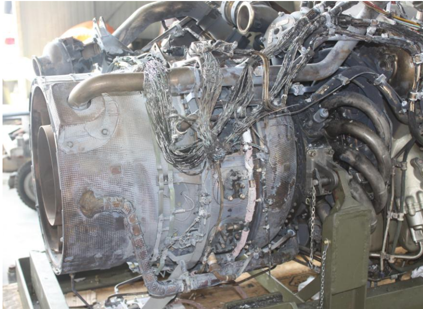
Figure 12: The evidence of fire on the external of hot section area
