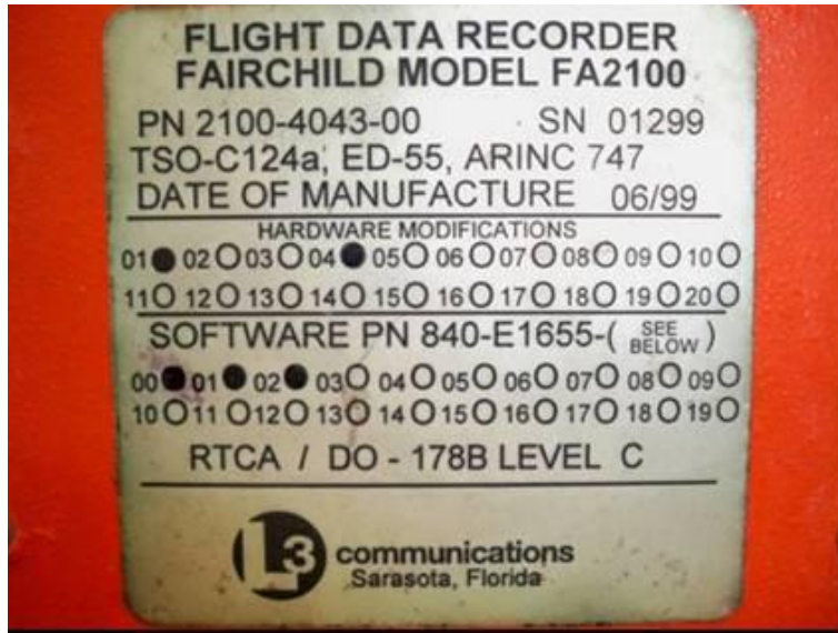
Figure 2: PK-YRP FDR identification plate
