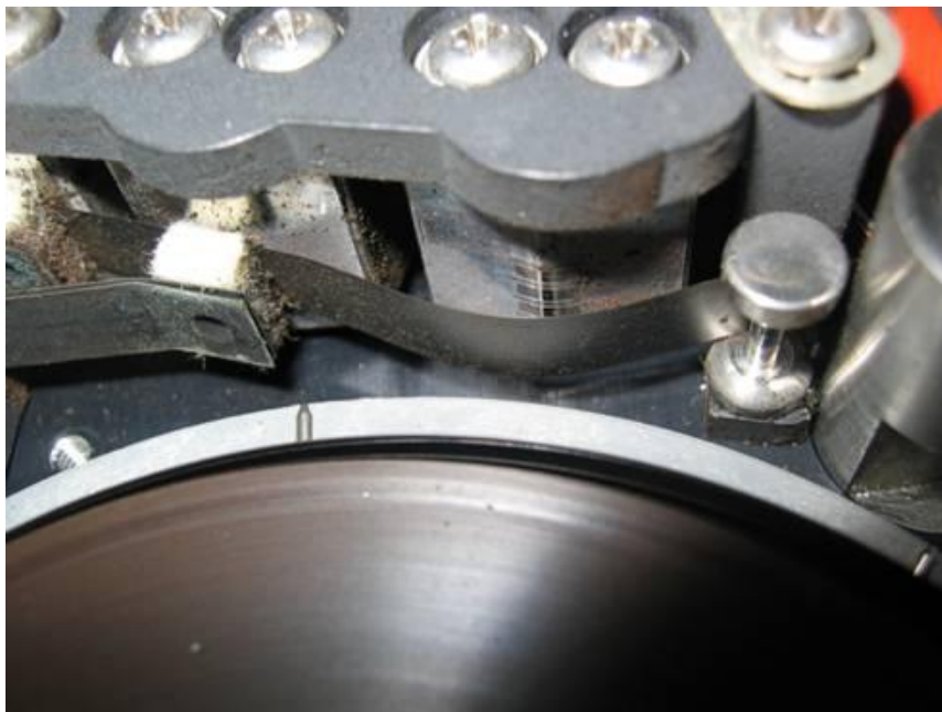
Figure 5: CVR recording head was worn-out and dirty
