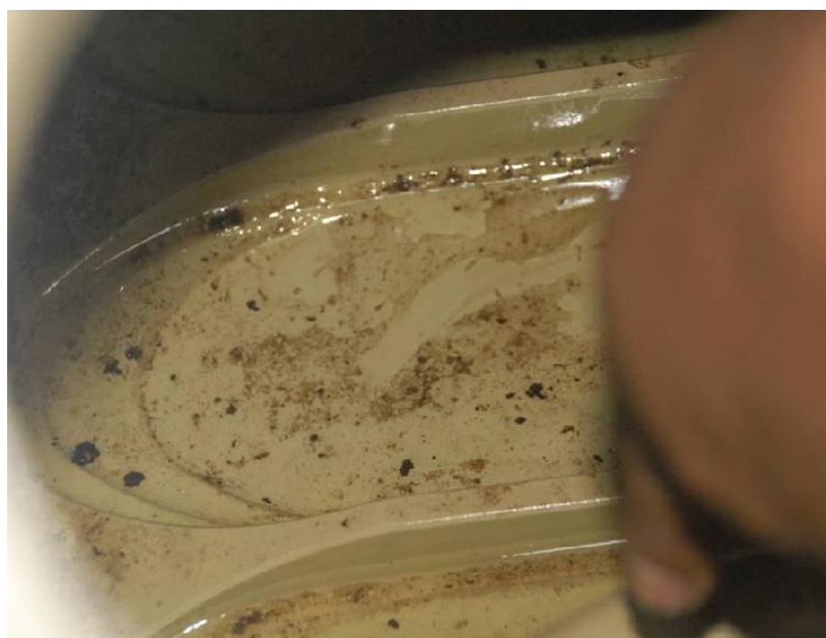
Figure 17: Uncured sealant and deposit
