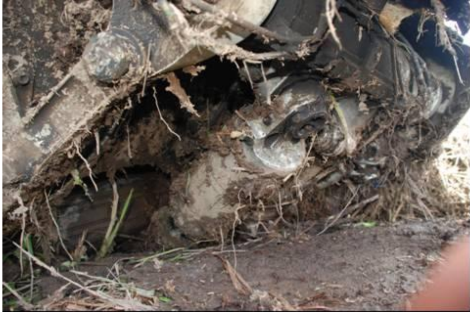
Figure 10: The right main landing gear was broken
