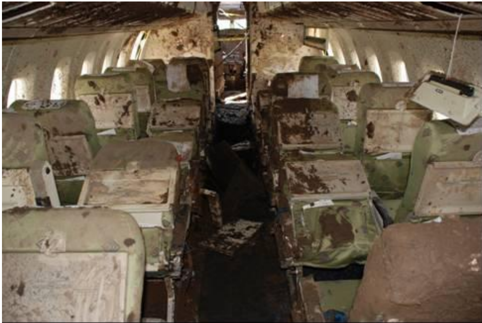
Figure 12: View of passenger cabin damage
