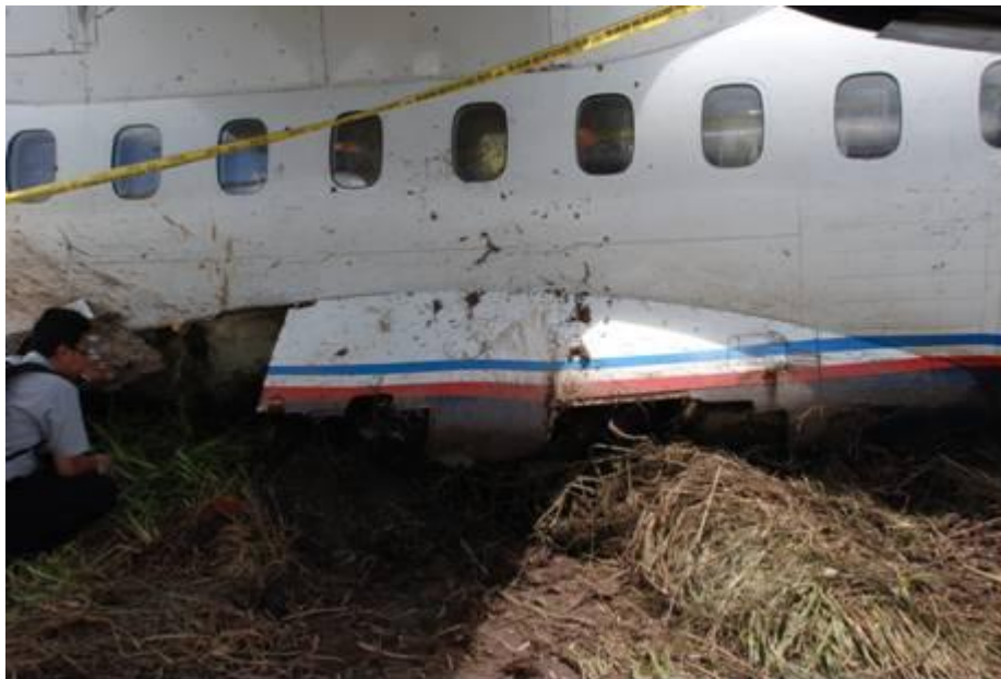
Figure 9: The right main landing gear door was broken
