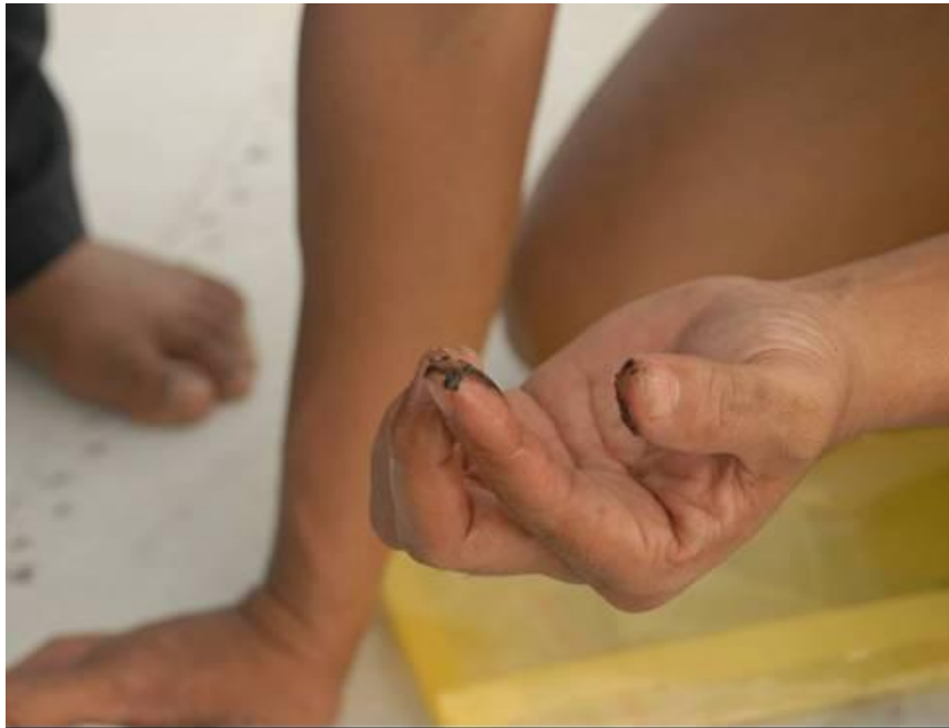
Figure 18: Uncured sealant from the wing tank
