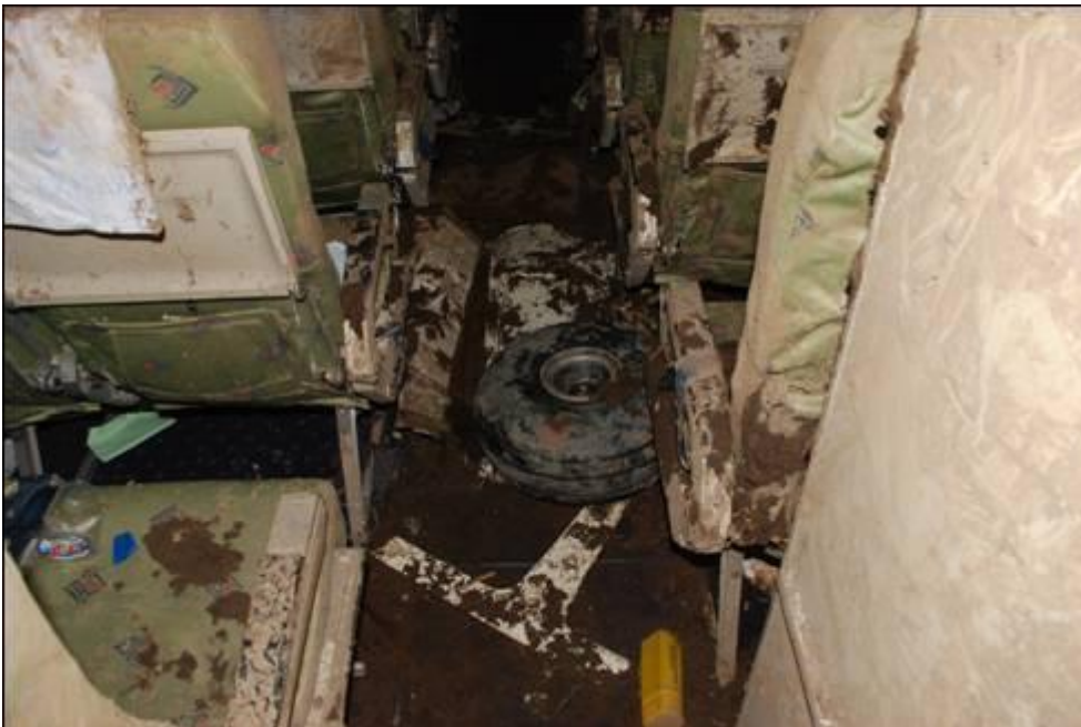
Figure 13: Nose wheel found inside the cabin
