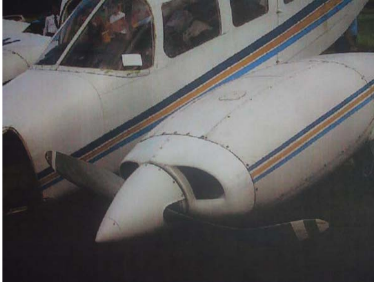
Figure 2: PK-SUV at accident site. Left engine propeller blades were bent
