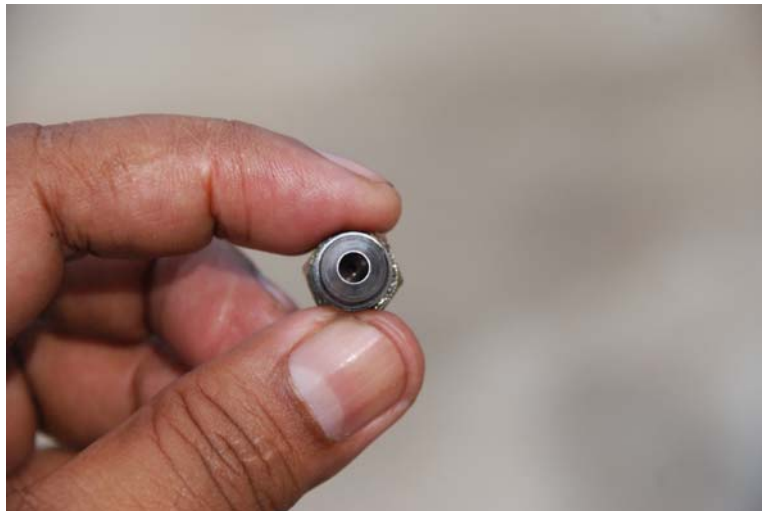
Figure 6: Hydraulic restrictor 0.31 diameter
