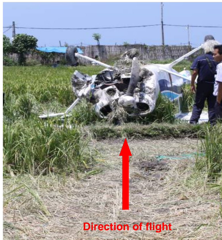
Figure 2: The aircraft's propeller and nose landing gear were damaged
