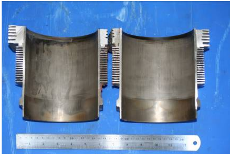
Figure 4: De-lamination of coating.
