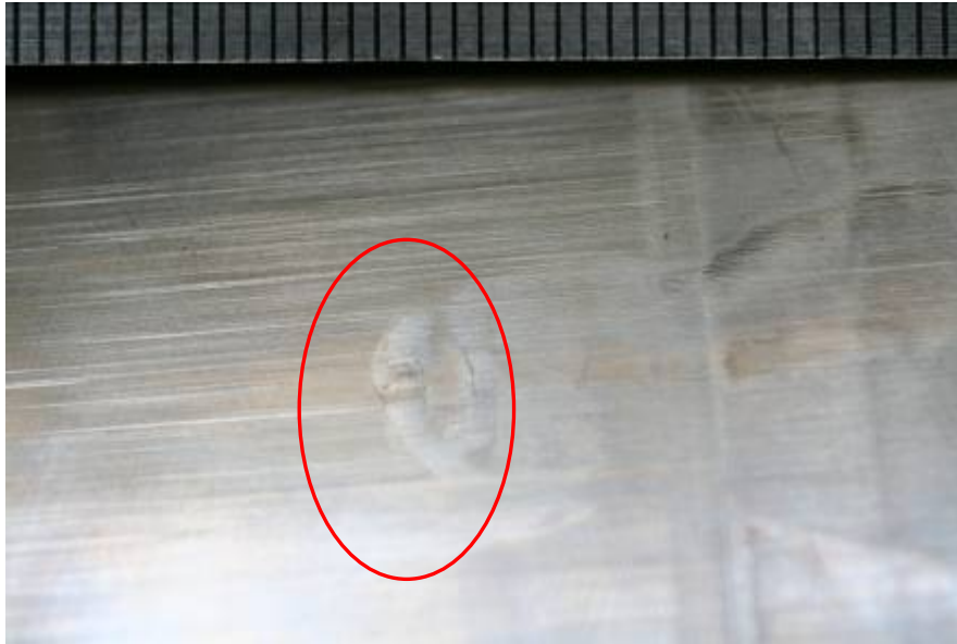
Figure 7: Blister of long type found near the BDC (Bottom Dead Centre). Cracks started to develop at the blister
