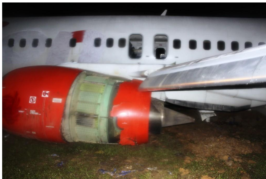
Figure 1: The damage of the left engine
