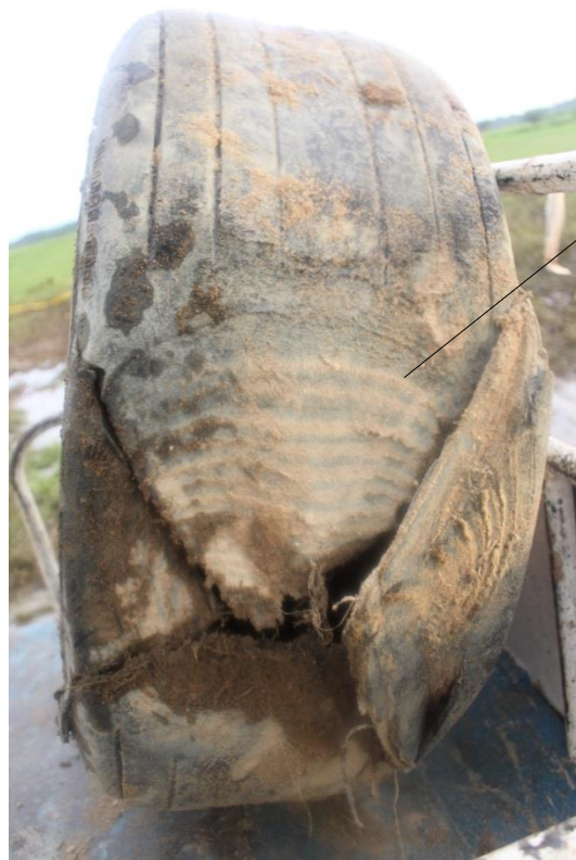
Figure 8: The number 3 tire ripped and scratched
