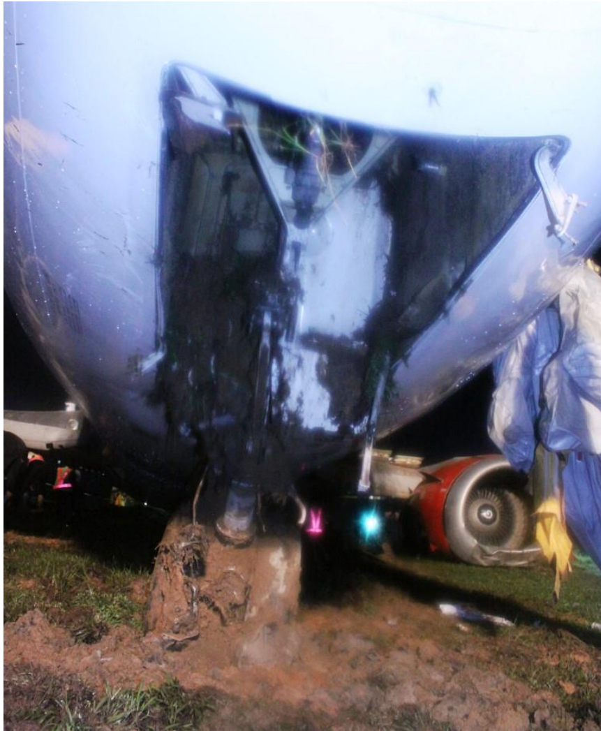
Figure 2: The damage on the nose landing gear
