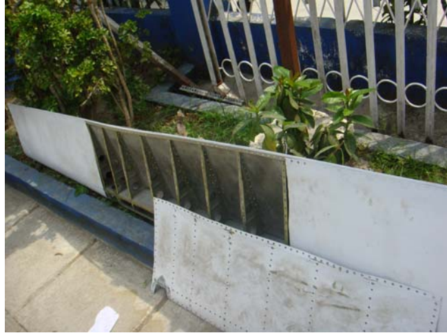
Figure 3: Lower skin of the right aileron scratched
