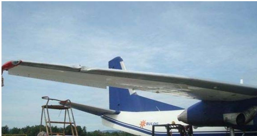
Figure 2: Damage on the right wing leading edge
