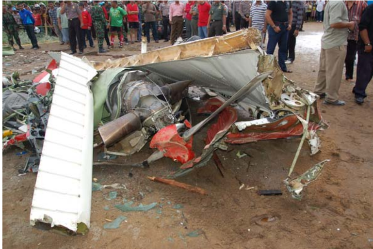
Figure 7: The Engine & Propeller damaged
