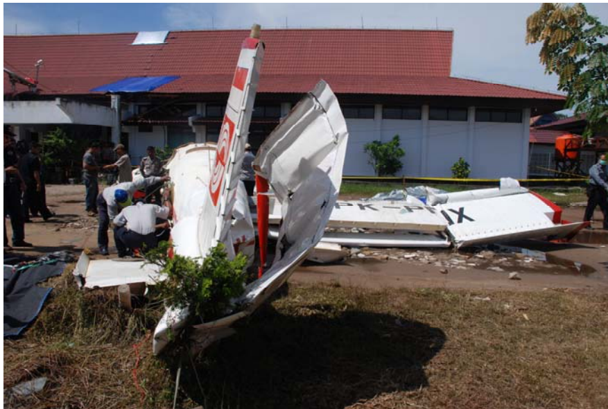
Figure 6: The tail section damaged
