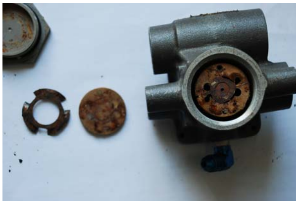
Figure 9: The Plate & Van pump was surface corrosion
