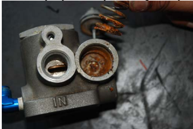
Figure 8: Booster Pump Pressure Regulator shown the spring was surface corrosion
