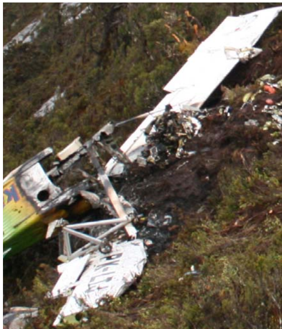
Figure 3: Destroyed forward fuselage and wings at the completion of on-site activities
