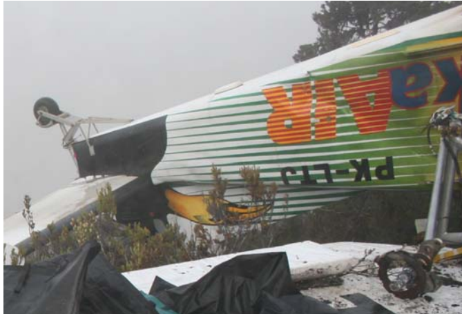
Figure 4: Inverted rear fuselage showing undamaged tail wheel
