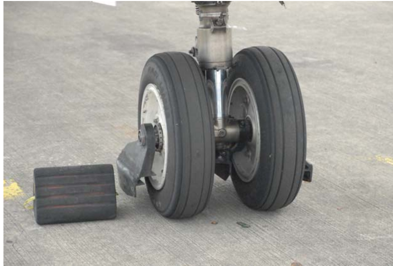
Figure 5: The association of wheel chuck to the ground clearance which usually used on nose gear during park, could cause the damage of the water deflector
