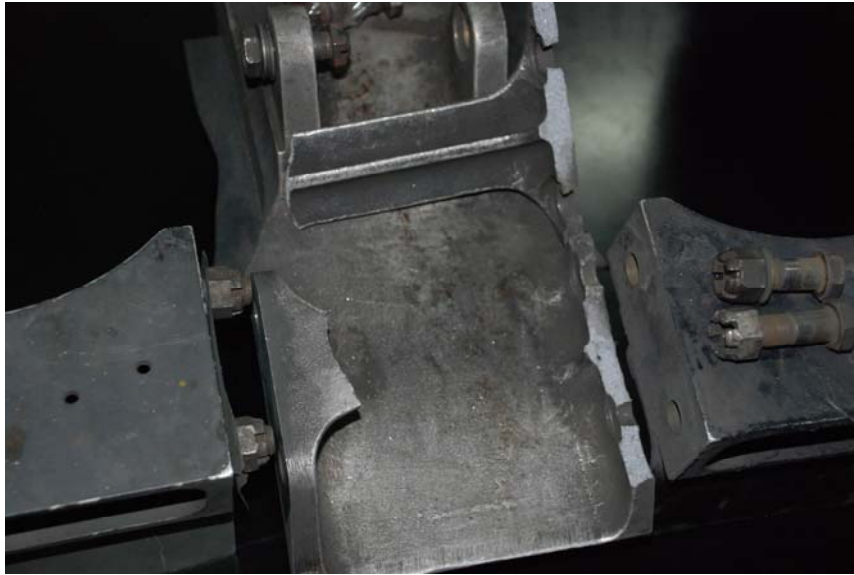
Figure 8: The broken attachment flange
