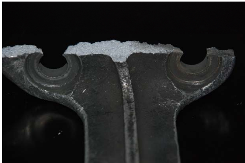
Figure 11: The flange hole edge was over-torque
