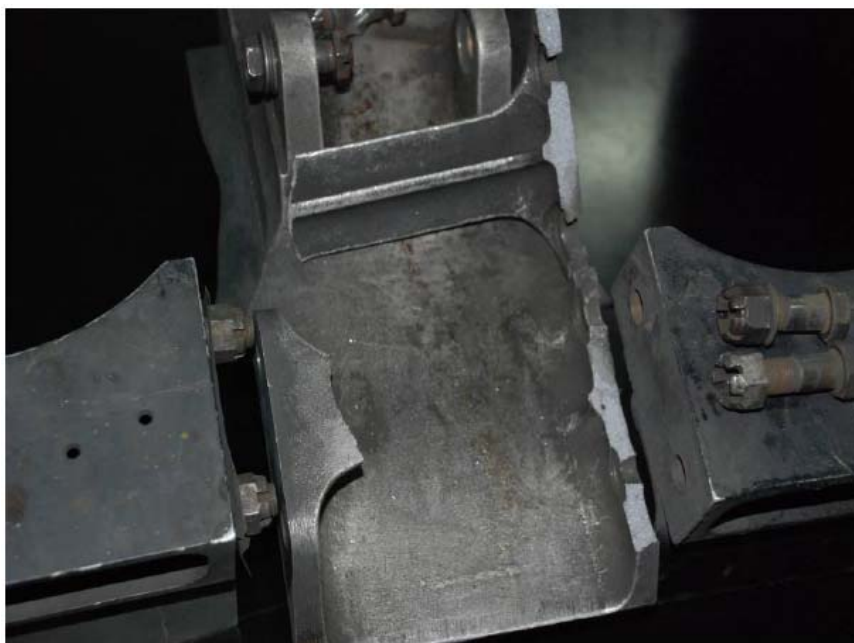
Figure 3: The fracture surface shows a dark colored portion indicating a pre-existing crack
