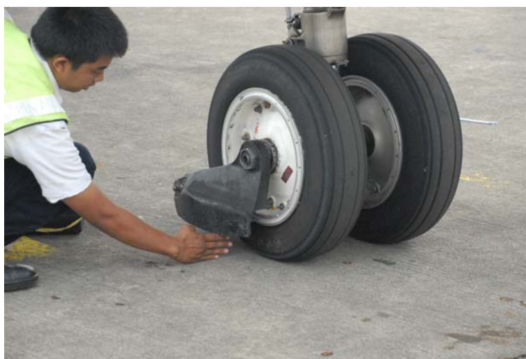
Figure 4: Showing the ground clearance of water deflector relative to the surface
