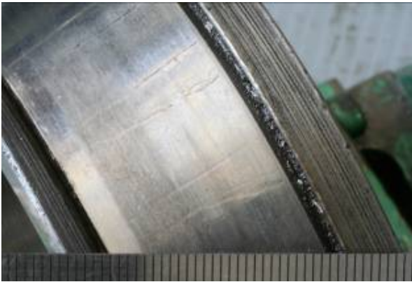
Figure 3: Roller impressions on the shiny surface of the inner raceway were indications of true Brinelling as a result of under torque.
