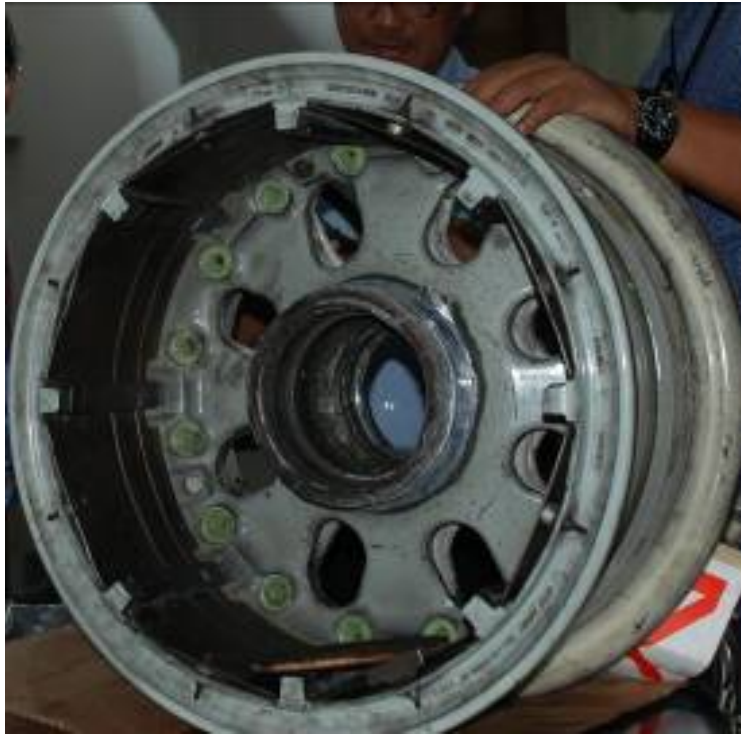
Figure 4: Number-two main wheel hub assembly after removal of the tire.
