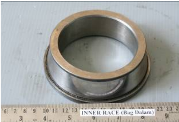
Figure 2: Shiny surface of the inner raceway of the inboard bearing
