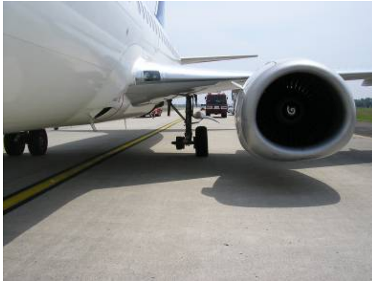
Figure 1: View after landing showing the number-two axle without wheel
