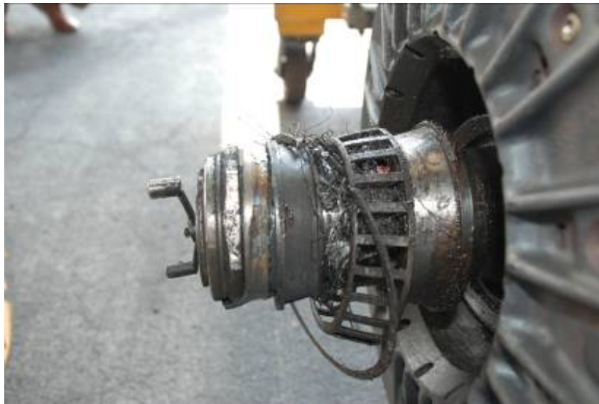
Figure 3: Damaged inner and outer wheel bearing race on number-two axle
