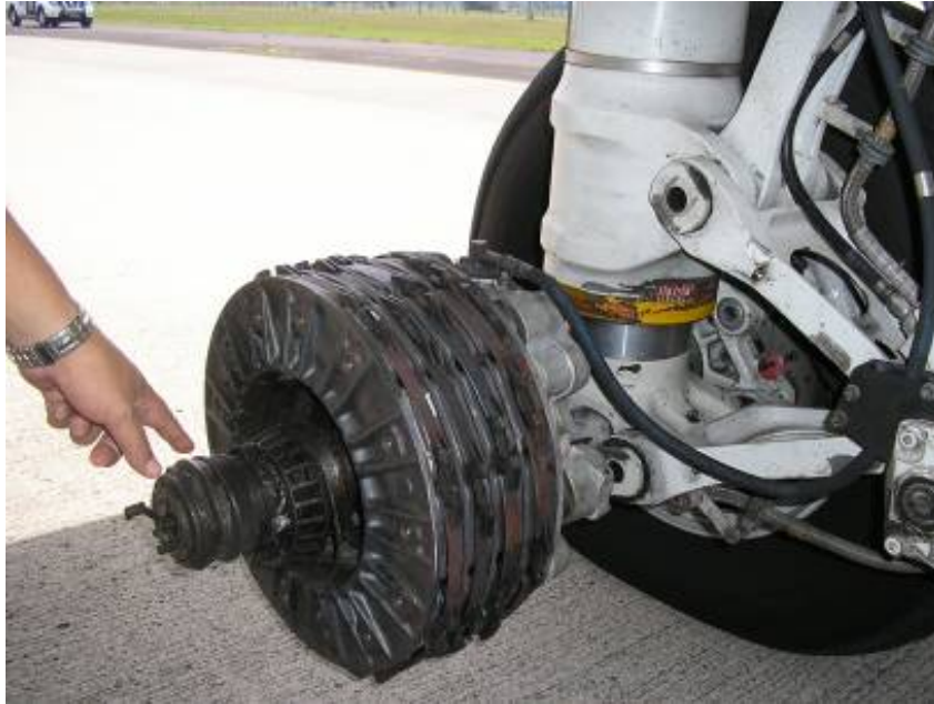
Figure 2: The number-two main wheel separated from its axle
