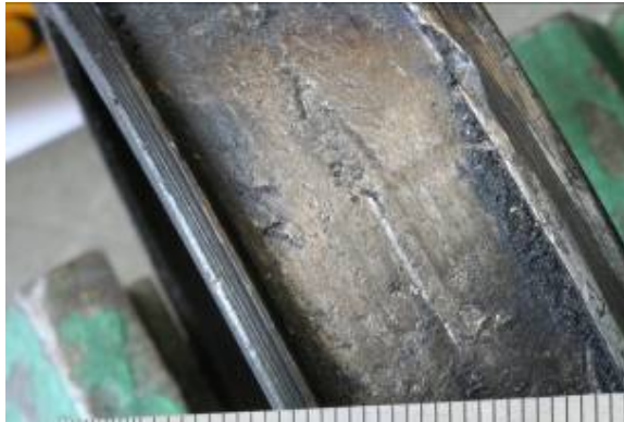
Figure 4: Dull surface on the inner raceway of the outboard bearing. Note the roller impressions indicating false Brinelling due to vibration.
