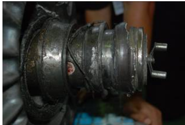
Figure 1: Bearing failures on the axle.
