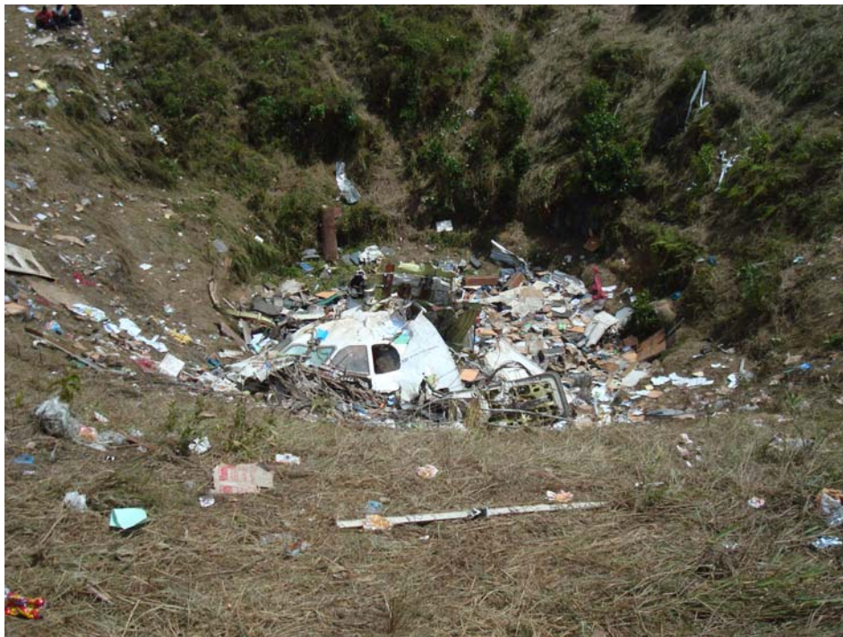
Figure 6: Cockpit section of PK-BRD
