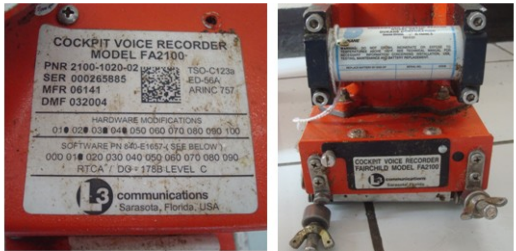
Figure 4: Data plate on Cockpit Voice Recorder from PK-BRD
