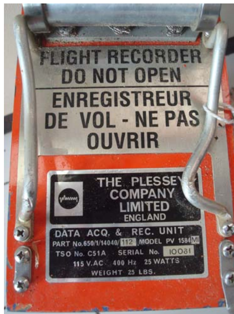
Figure 3: Data plate on Flight Data Recorder from PK-BRD
