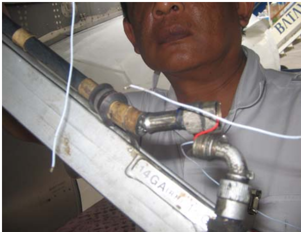
Figure 5: Broken left landing gear down lock cable
