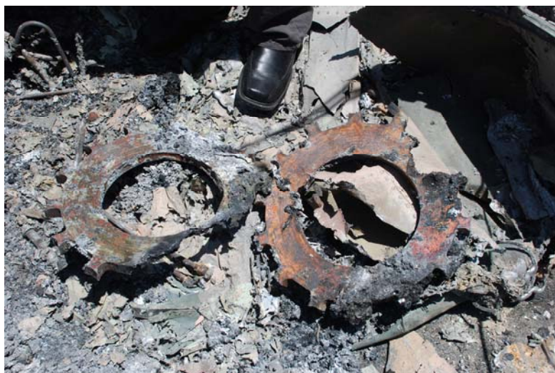
Figure 10: Left main landing gear aft brake inner and outer discs
