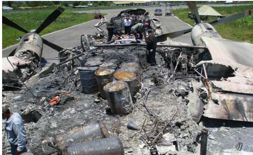
Figure 2: Burnt general freight, including diesoline and turbine fuel in drums
