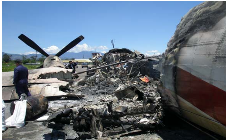
Figure 8: The fire started in the left wheel bay. The wings collapsed onto the main wheel area
