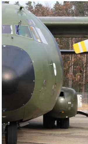
Figure 12: View of a Transall C-160 main landing gear. Note the wheels covered by the landing gear bay
