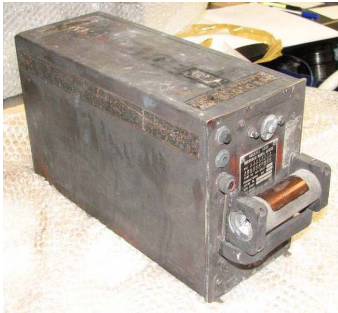
Figure 5: Fire damaged Cockpit Voice Recorder box
