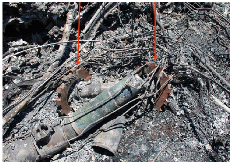
Figure 9: Arrows point to left main landing gear, front brake outer and inner discs. Right arrow also indicates hydraulic lines
