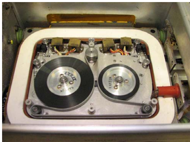
Figure 4: Undamaged contents of Universal Flight Data Recorder
