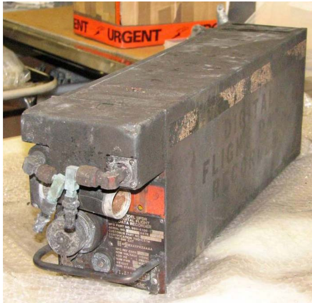
Figure 3: Fire damaged Universal Flight Data Recorder box
