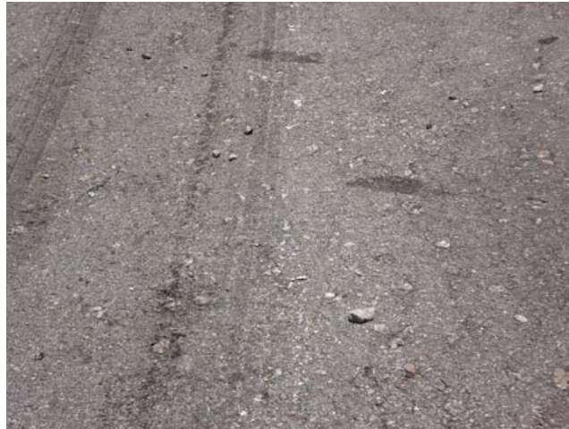
Figure 7: Molten metal on the runway in the aircraft's wheel tracks
