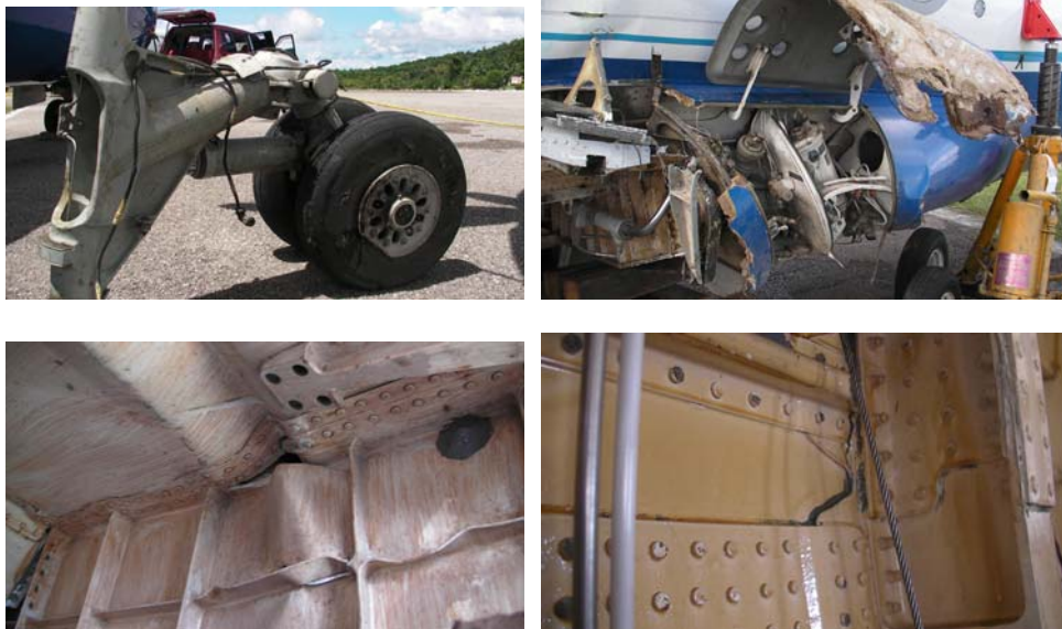
Figure 4: Damaged left main landing gear, landing gear bay, and left fuselage structure
