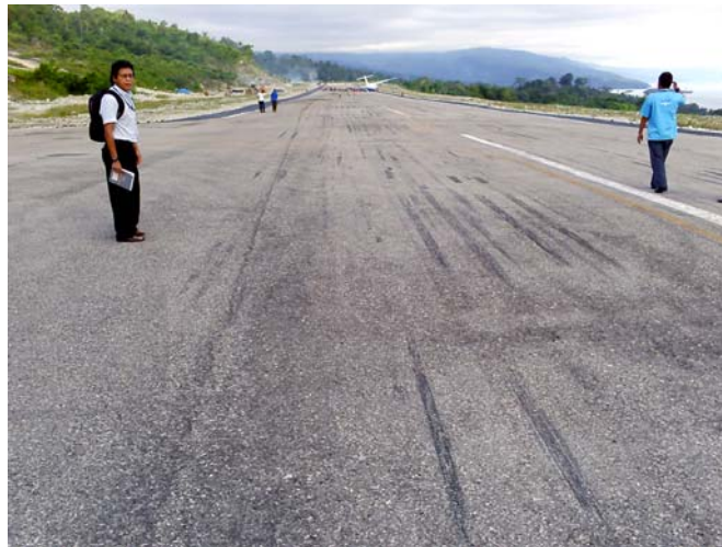
Figure 3: Left wheel mark from PK-TXL on the runway approximately 100 meters from the touch-down end of the runway.
