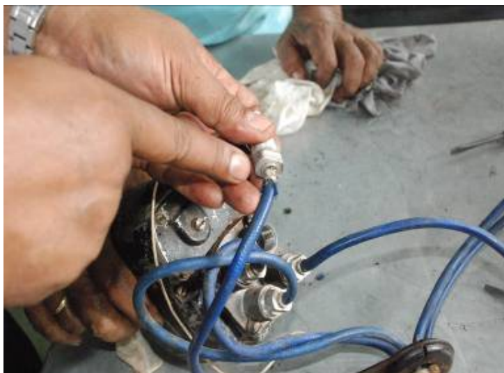
Figure 6: The left magneto harness broken
