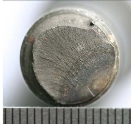
Figure 4: Bolt C; Fracture surface with a fatigue crack of 11mm long. (circumferentially)
