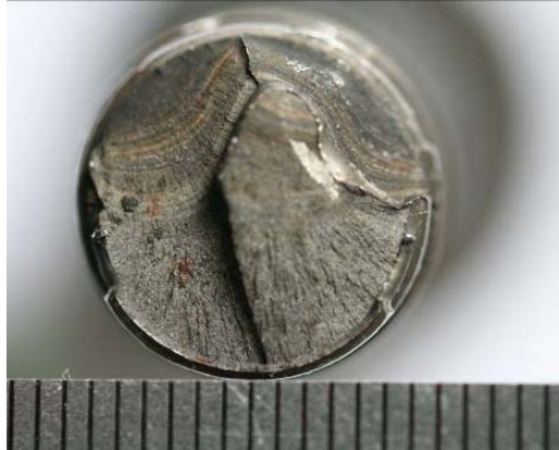
Figure 3: Bolt B; Fracture surface with a fatigue crack of 14mm long. (circumferentially)
