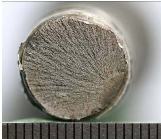
Figure 5: Bolt A: Fracture surface with a fatigue crack of 7mm long (circumferentially).
