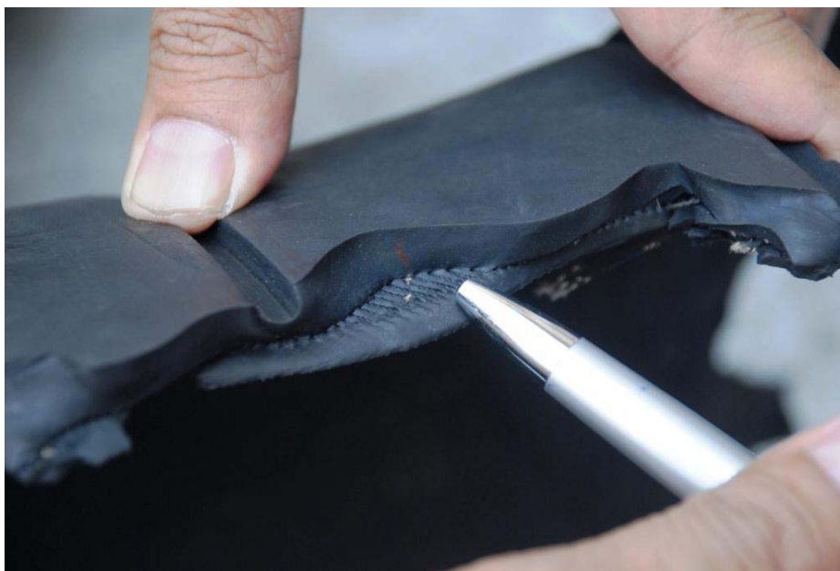
Figure 9: The shape of the cut and the nylon holes are not types of damage by FOD.
