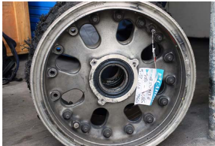
Figure 2: Wheel number-1 hub with four of sixteen bolts that were broken
