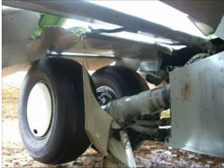
Figure 1: Right landing gear collapsed rearward
