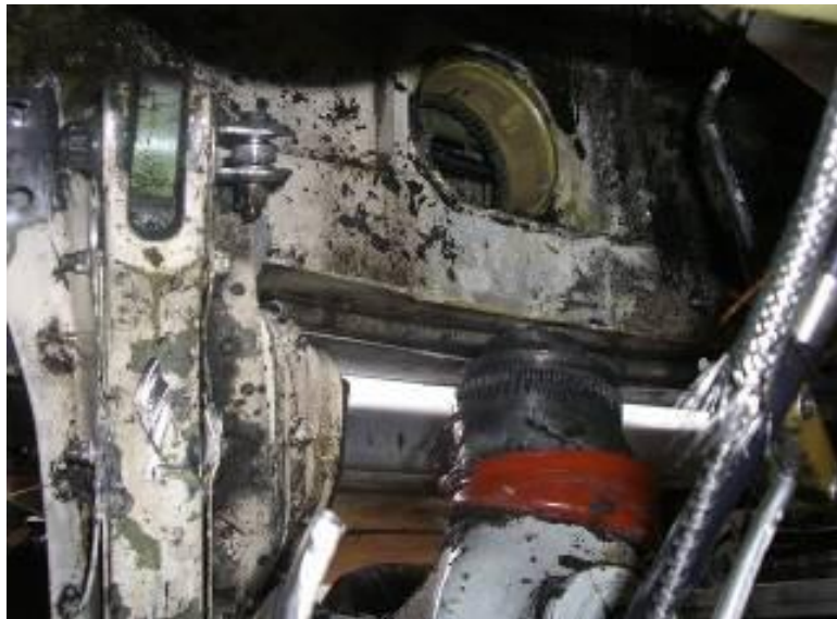
Figure 2: Detached right main landing gear retraction axle
