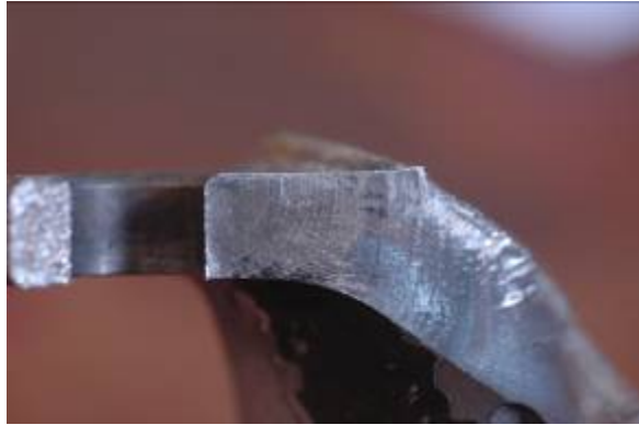
Figure 4: Beach marks on the fracture surface.
