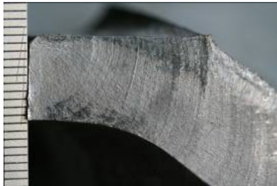
Figure 5: Beach marks propagating from the hole edge
