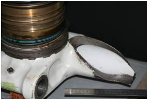
Figure 1: The fractured axle of the number-one main landing gear
