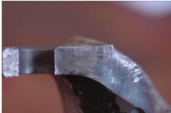
Figure 4: Beach marks on the fracture surface.
