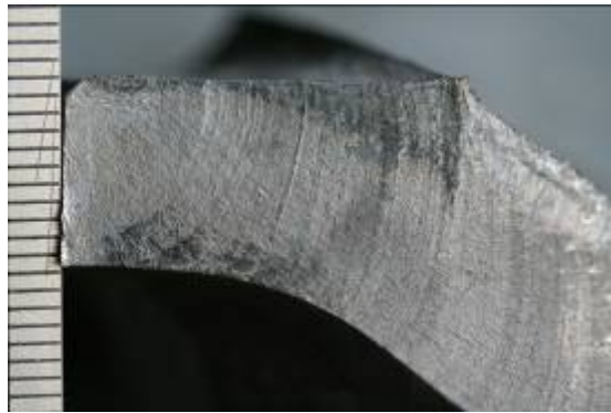
Figure 5: Beach marks propagating from the hole edge
