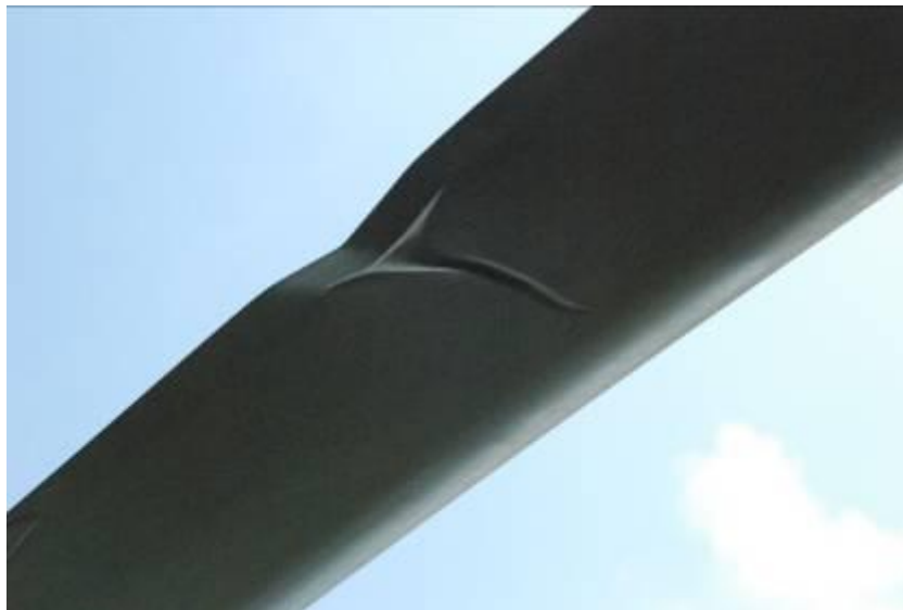
Figure 11: The main rotor blade trailing edge was bent caused impact
