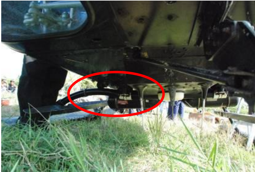
Figure 6: The forward right skid was bent
