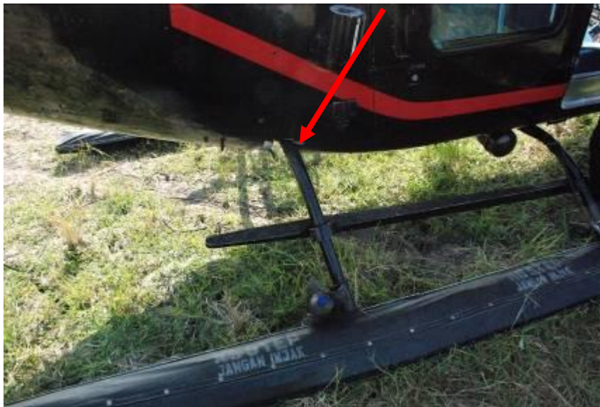
Figure 7: Aft right skid was bent
