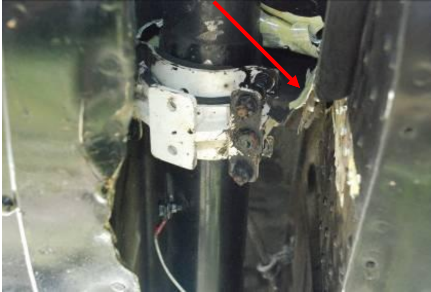
Figure 8: The fwd right attachment skid torn and detached
