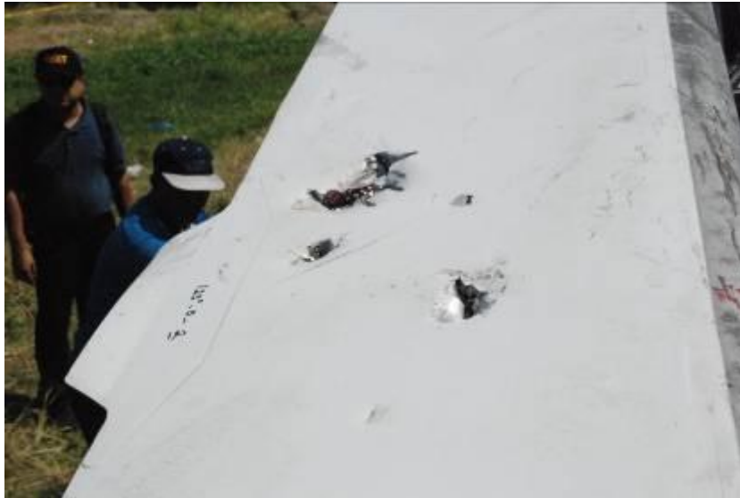
Figure 10: The main rotor blade surface marking caused impact to the ground
