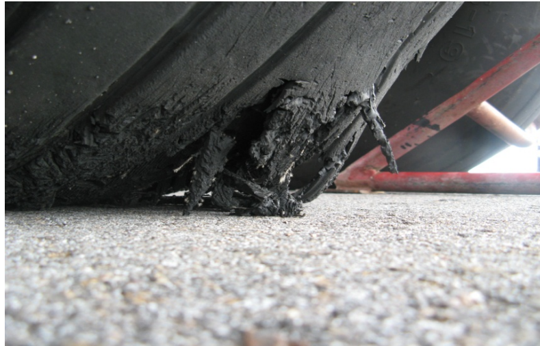
Figure 4: Tire number three was substantially damaged
