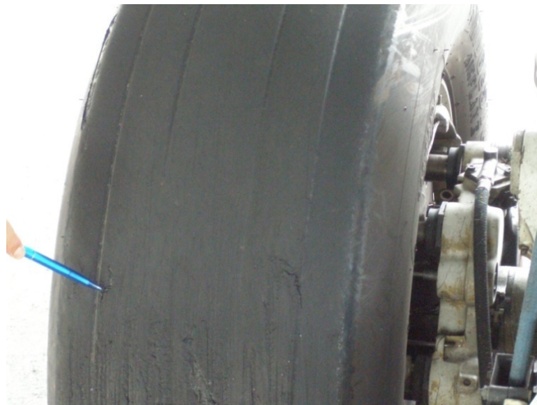
Figure 5: Damaged tire number two
