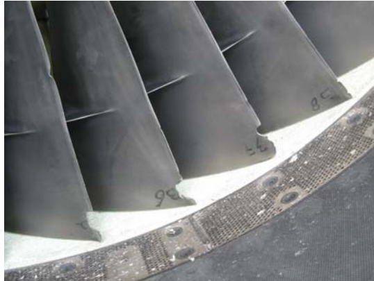
Figure 6: Damaged engine fan blades
