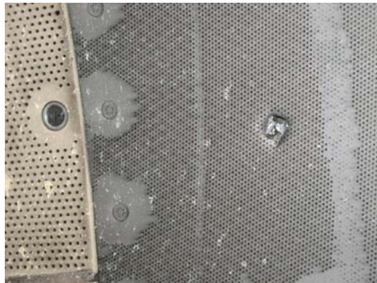
Figure 7: Damaged number-two engine air intake screen
