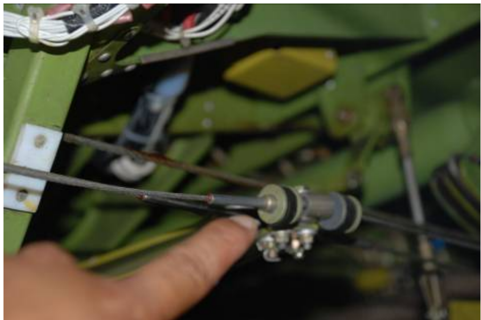
Figure 7: Rudder cable tension slackened from structural damage at impact
