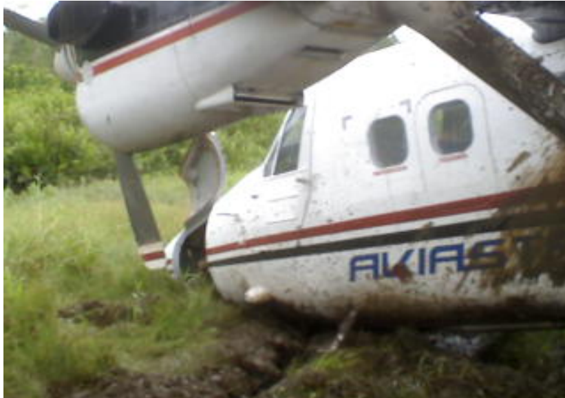
Figure 4: Forward fuselage and nose landing gear buried in soft ground
