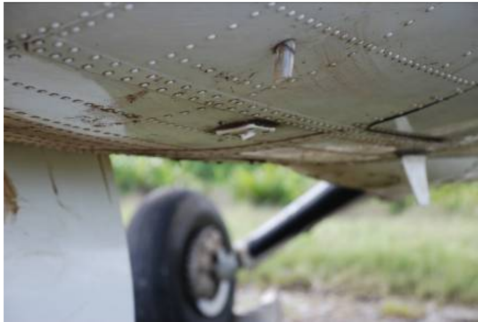
Figure 6: Broken ADF antenna
