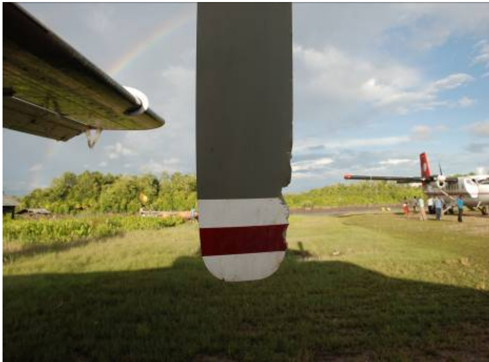
Figure 8: One damaged left propeller blade
