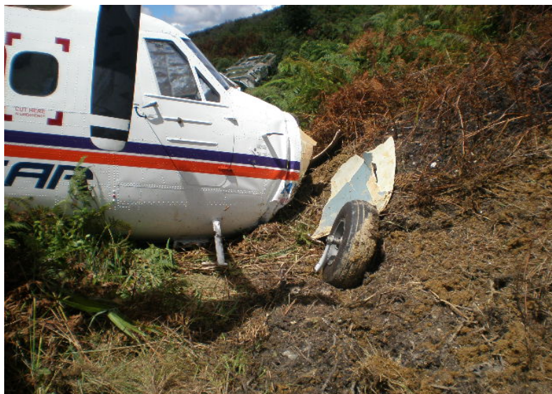
Figure 6: Nose and nose landing gear damage
