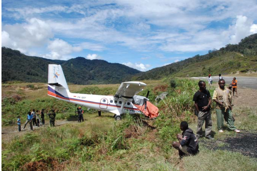
Figure 2: Aircraft after impact with the embankment
