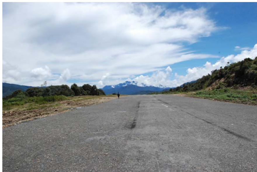
Figure 3: Nose wheel and left wheel marks of skidding to the left, starting from touch down point
