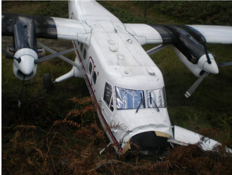
Figure 5: View showing aircraft nose damage
