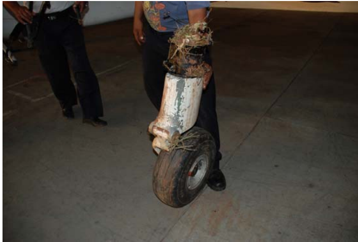
Figure 6: The nose wheel was damaged
