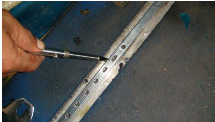
Figure 8: The hole rail to inserted the pin
