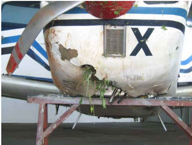
Figure 5: The lower engine cowling condition after occurrence
