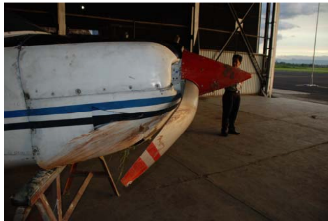
Figure 3: One of the propellers was dent
