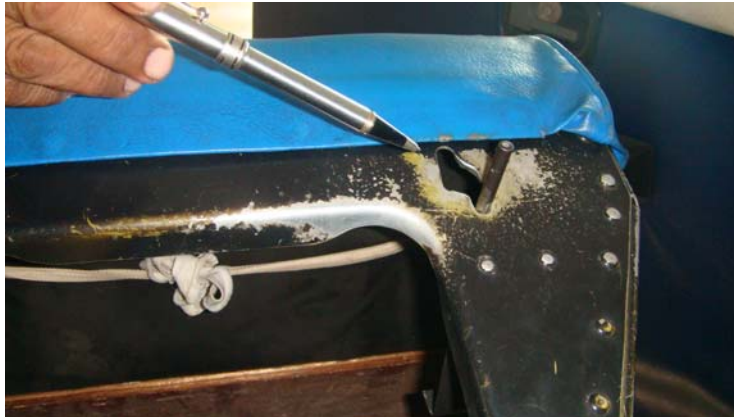
Figure 9: The locking handle to moved the seat forward and backward
