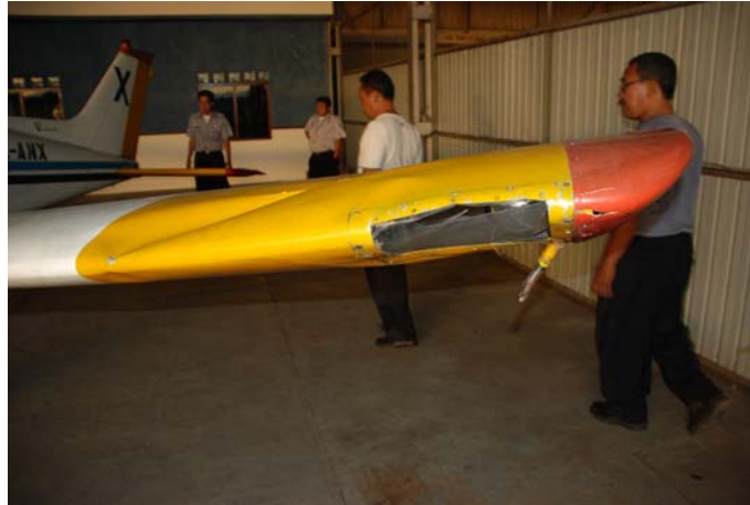
Figure 2: The left wing was dent and the wing tip was broken
