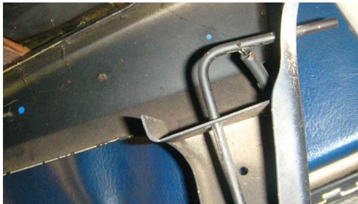
Figure 10: The spring in the locking handle
