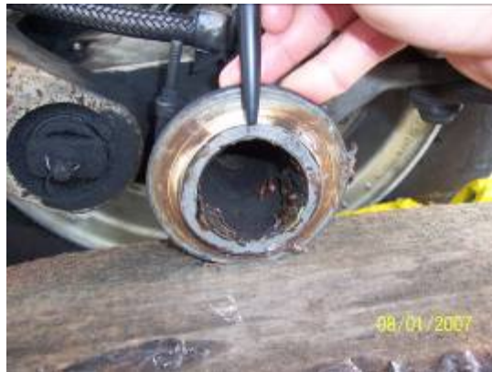
Figure 2: Damaged on the right nose wheel axle shaft
