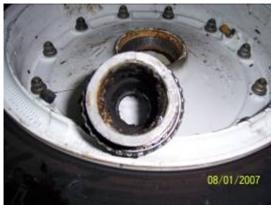
Figure 3: The right nose wheel axle shaft and the right nose wheel
