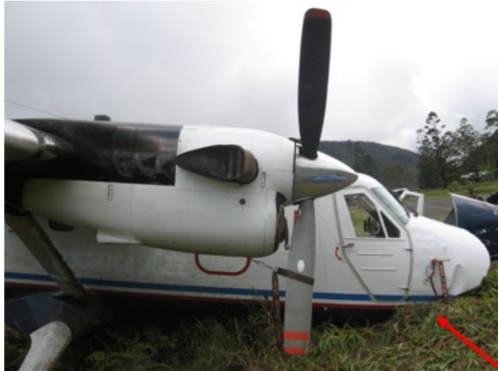
Figure 5 : Nose landing gear area indicated by arrow
