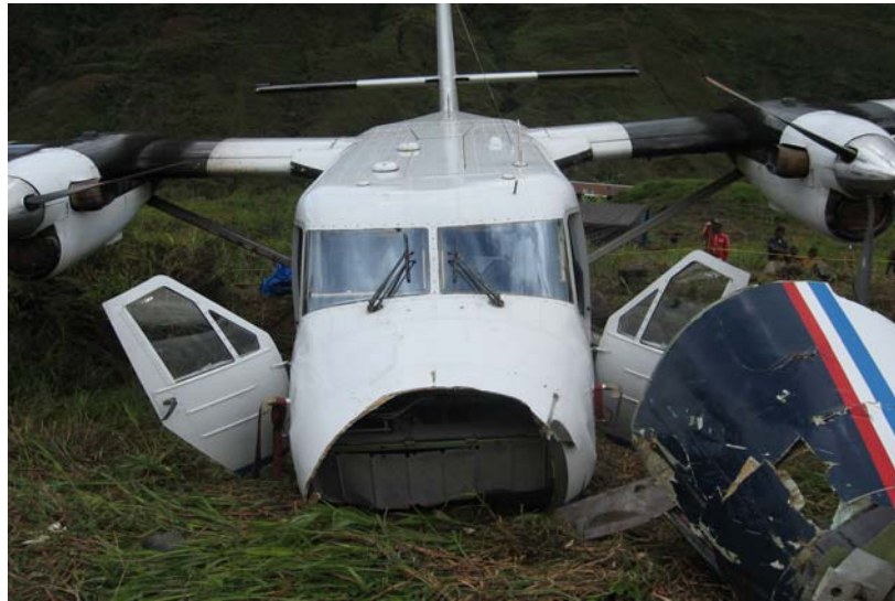
Figure 3 : Forward fuselage substantially damaged
