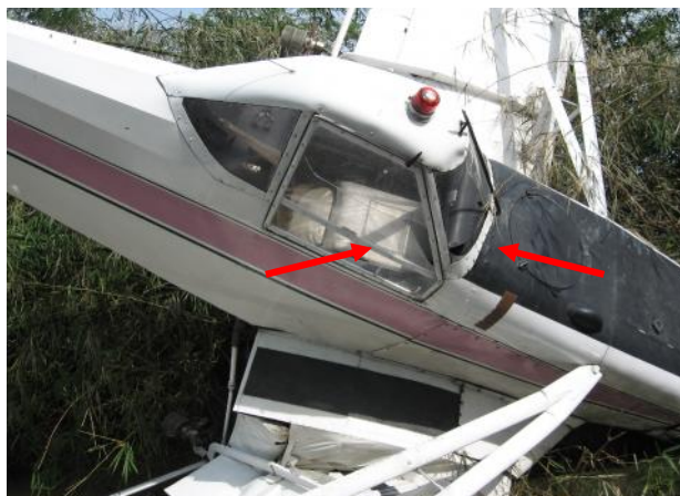
Figure 4: The broken windshield
