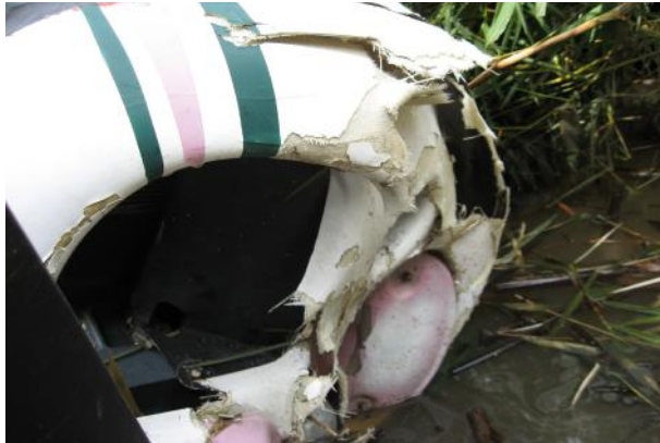
Figure 5: Bamboo pieces in the engine cowling
