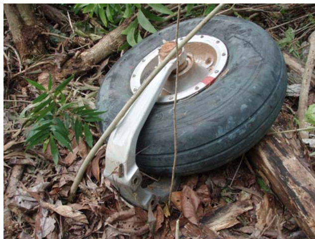
Figure 2: Severed nose landing gear
