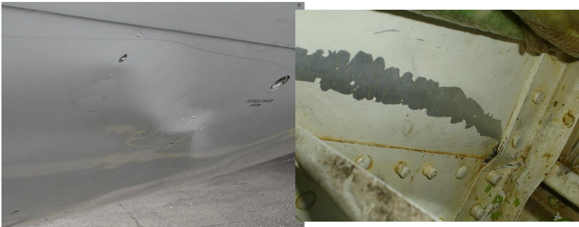
Figure 1: wrinkle of the fuselage skin and structure damage on the nose landing gear area
