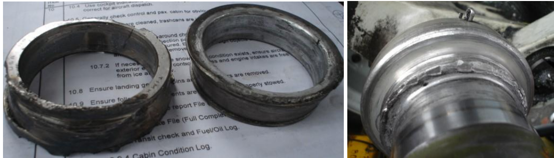
Figure 2: damage on the left main landing gear axle and bearing
