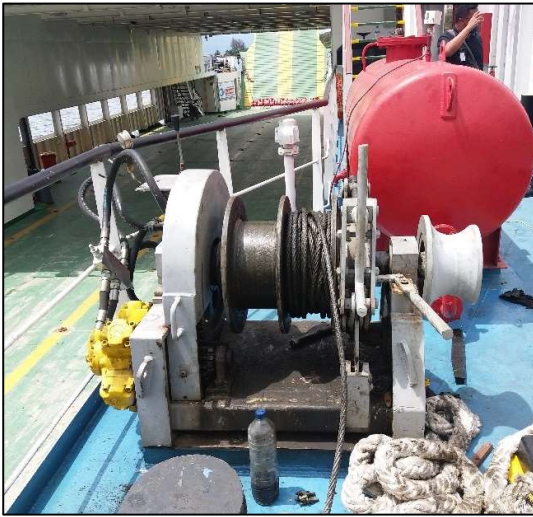
Gambar 4: Hydraulic winch pintu rampa buritan
