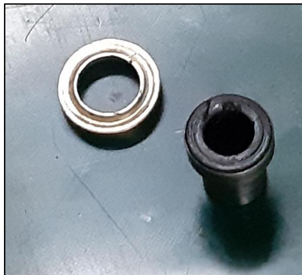
Figure II-3: The close-up view of broken rubber and brass parts
