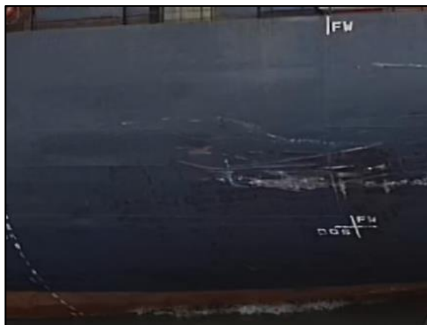
Figure I-16: Scratch on the Soul Of Luck's aft port side hull
