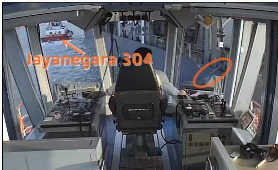
Figure I-7: Tug line of Jayanegara 201 (orange circle) was ready; Jayanegara 304 's was still not ready (source: CCTV footage of Jayanegara 201 )
