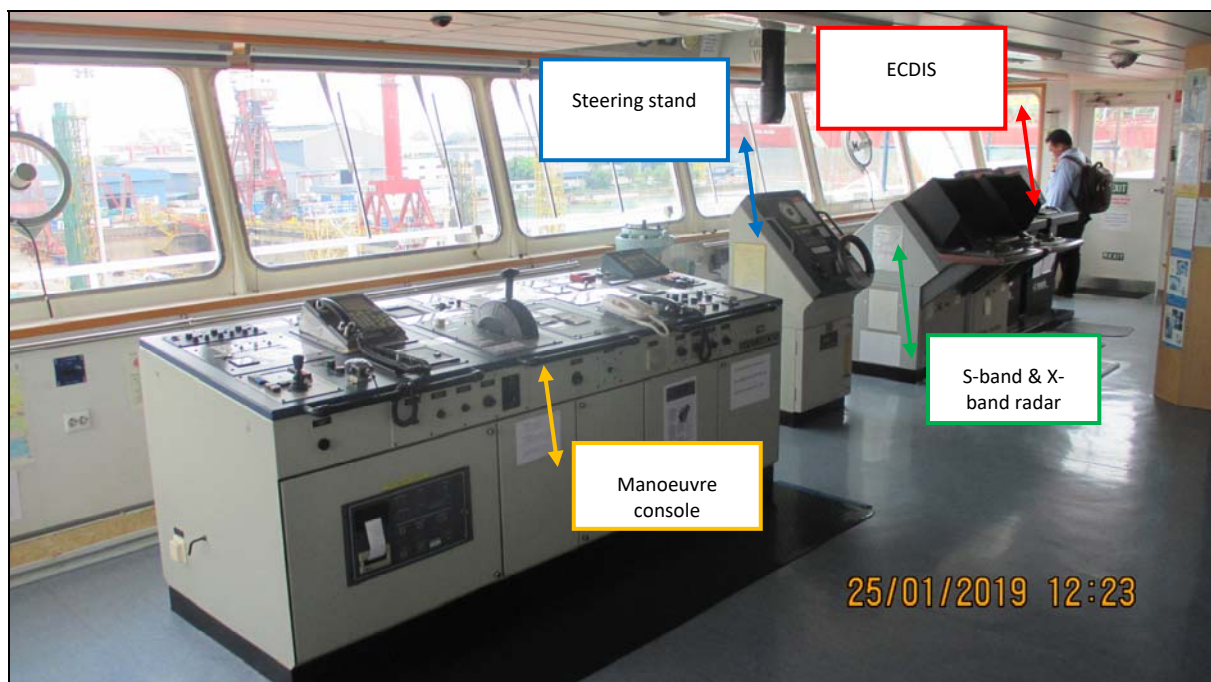
Figure I-23: Bridge layout on Antea
