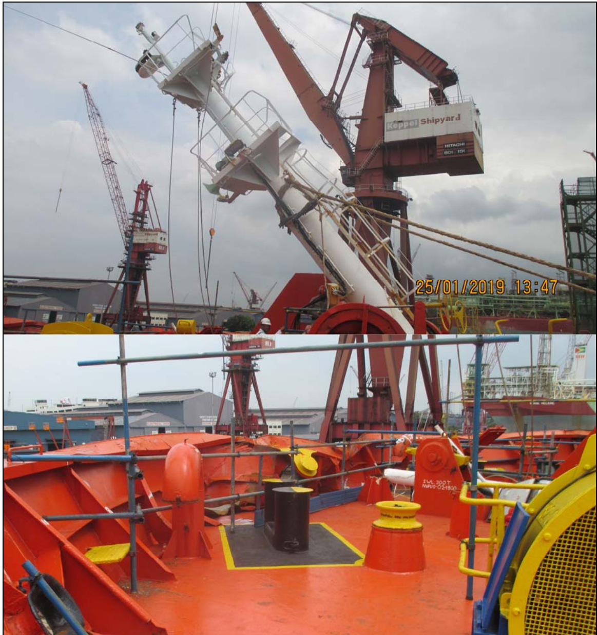
Figure I-19: Forecastle damage. Antea in Keppel dry dock
