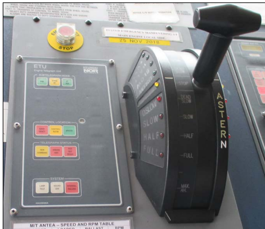
Figure I-25: The bridge engine telegraph unit
