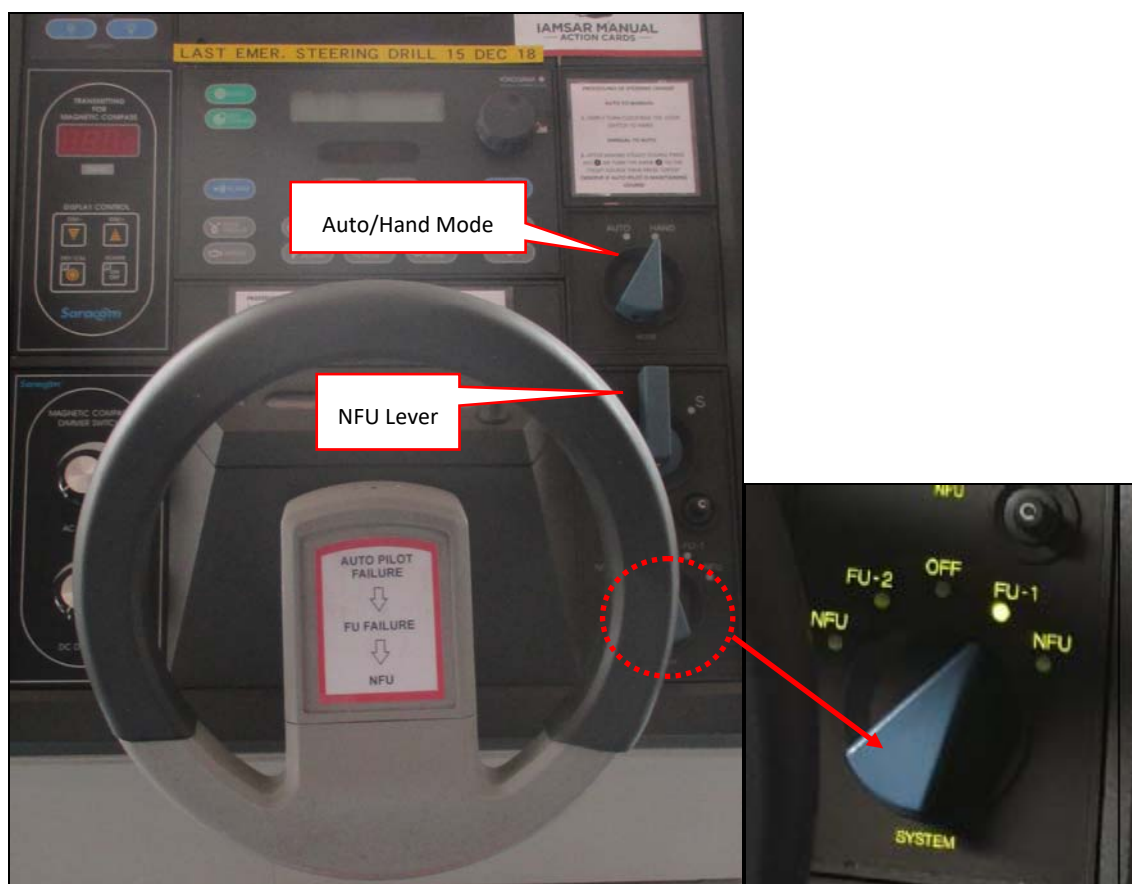
Figure I-24: Autopilot and wheel control on Antea
