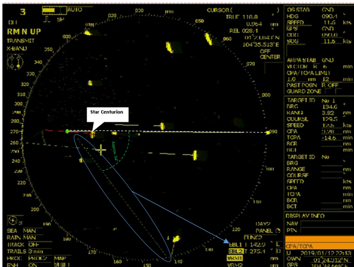
Figure II-1: Extract from X-band radar on Antea at 06:13:37 hours. The AB inform to the OOW that there was no response after he applied the steering to starboard
