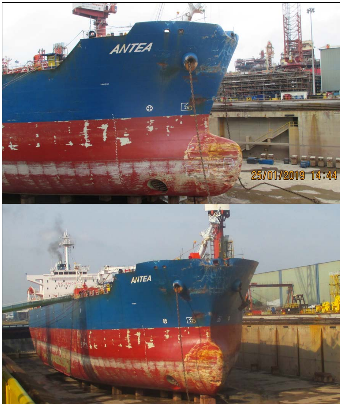
Figure I-18: Bow damage. Antea in Keppel dry dock
