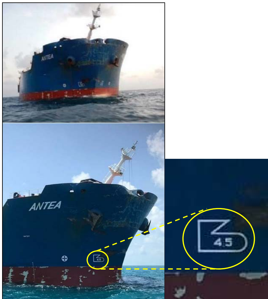
Figure I-17: Bow damage. Antea afloat following the collision
