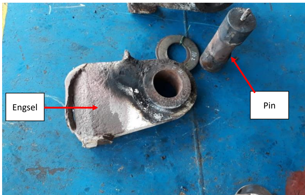
Gambar I-4: Engsel No.2 pintu rampa buritan
