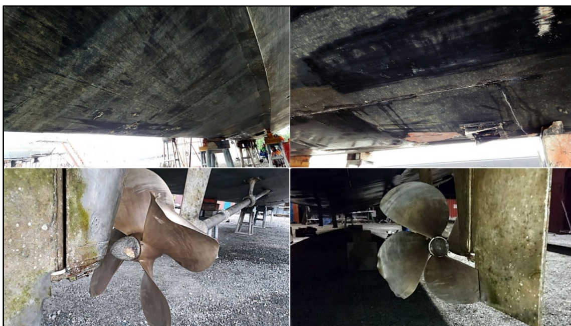
Figure 8: The damage profile of bottom plates and starboard propeller after Sea Flyte ran aground
