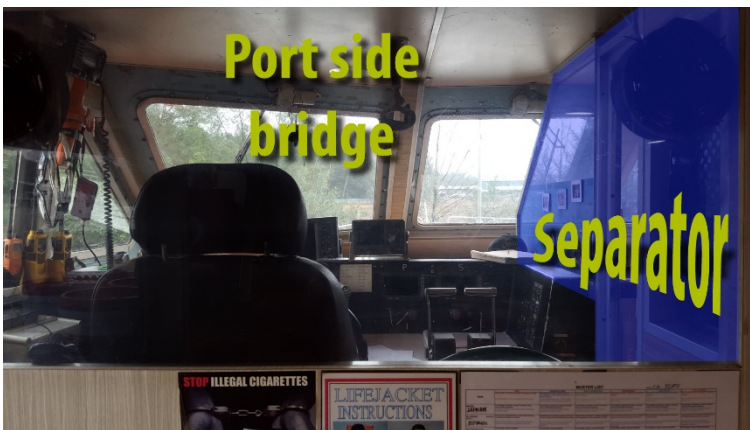
Figure 9: Starboard and port side bridge was separated by a wall
