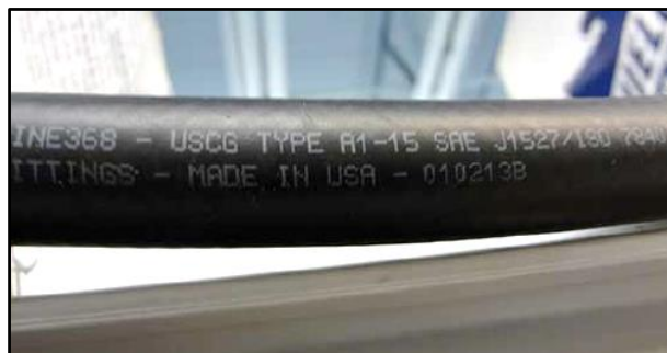
Gambar 12: Contoh marine fuel line tipe A1 standar USCG
