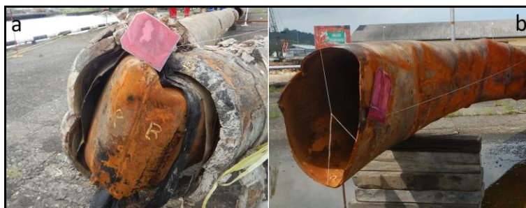
Figure I-16: a) A folded; and b) bent and cut subsea 20-inch pipe
