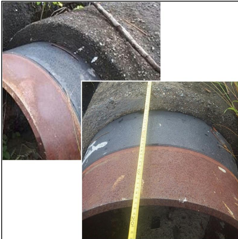
Figure I-33: Protection layers of an underwater pipe
