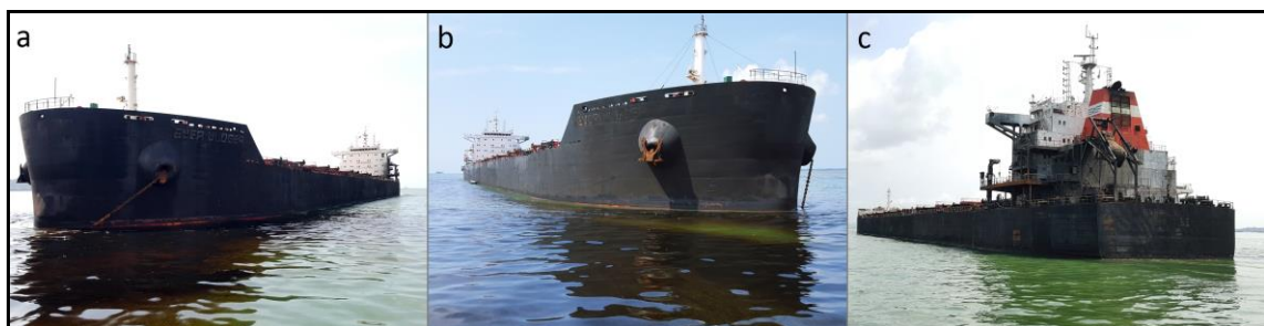
Figure I-7: The sooted hull of Ever Judger on P/S of her bow (a), S/B of her bow (b) and P/S of her aft
