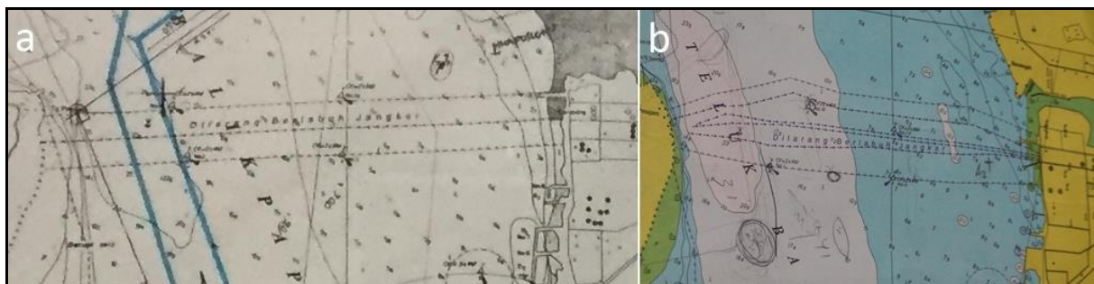
Figure I-28: Subsea pipes in Balikpapan Bay on the old (a) and new (b) marine chart
