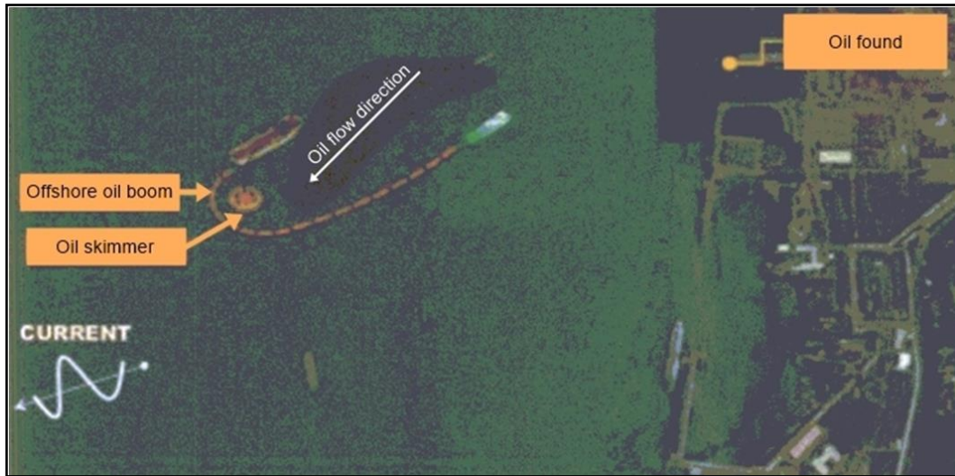
Figure I-24: J-formation in an oil spill drill in April 2017 (source: Pertamina RU V)
