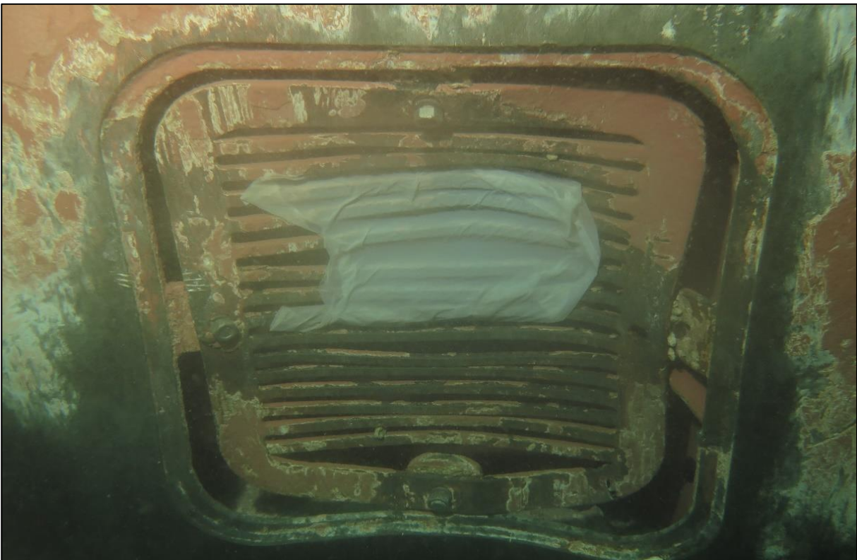
Gambar I-5: Kotak laut (sea chest) kisi-kisi bengkok
