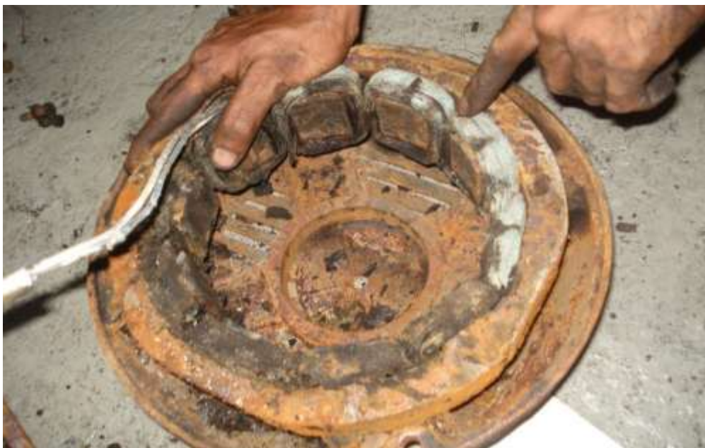
Gambar I-38: Pemeriksaan stator exciter KM. Zahro Express di workshop
