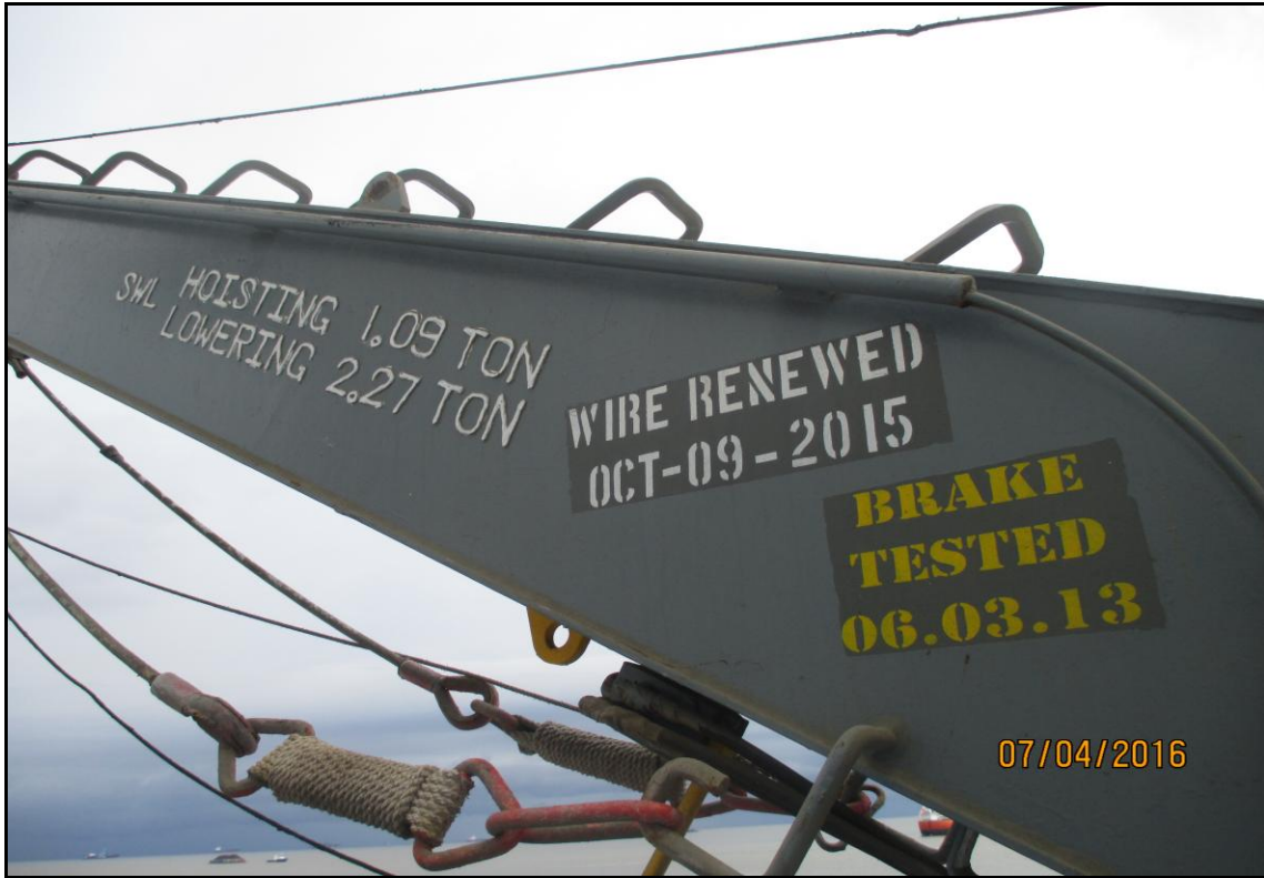
Figure I-14: Davit marked with the last wire replacement
