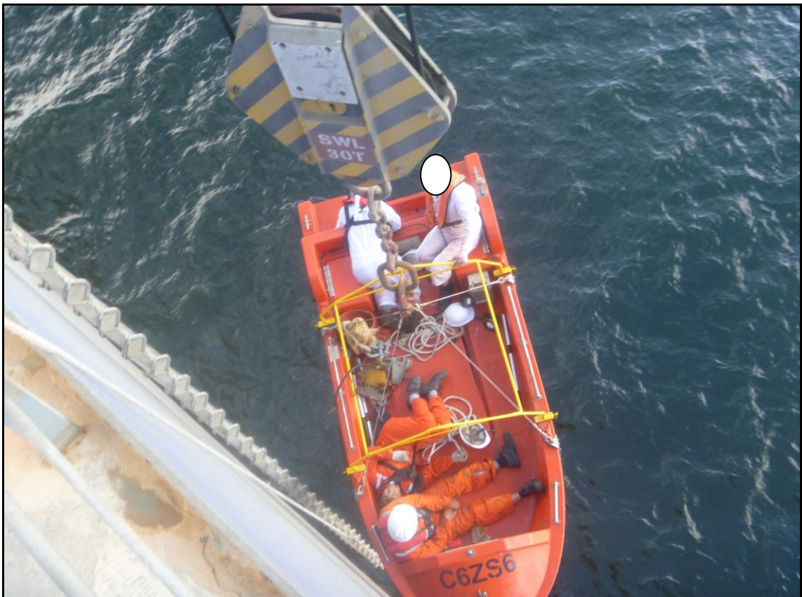
Figure I-12: Rescue boat hoisted by crane no.4 (picture taken by the ship's crew)
