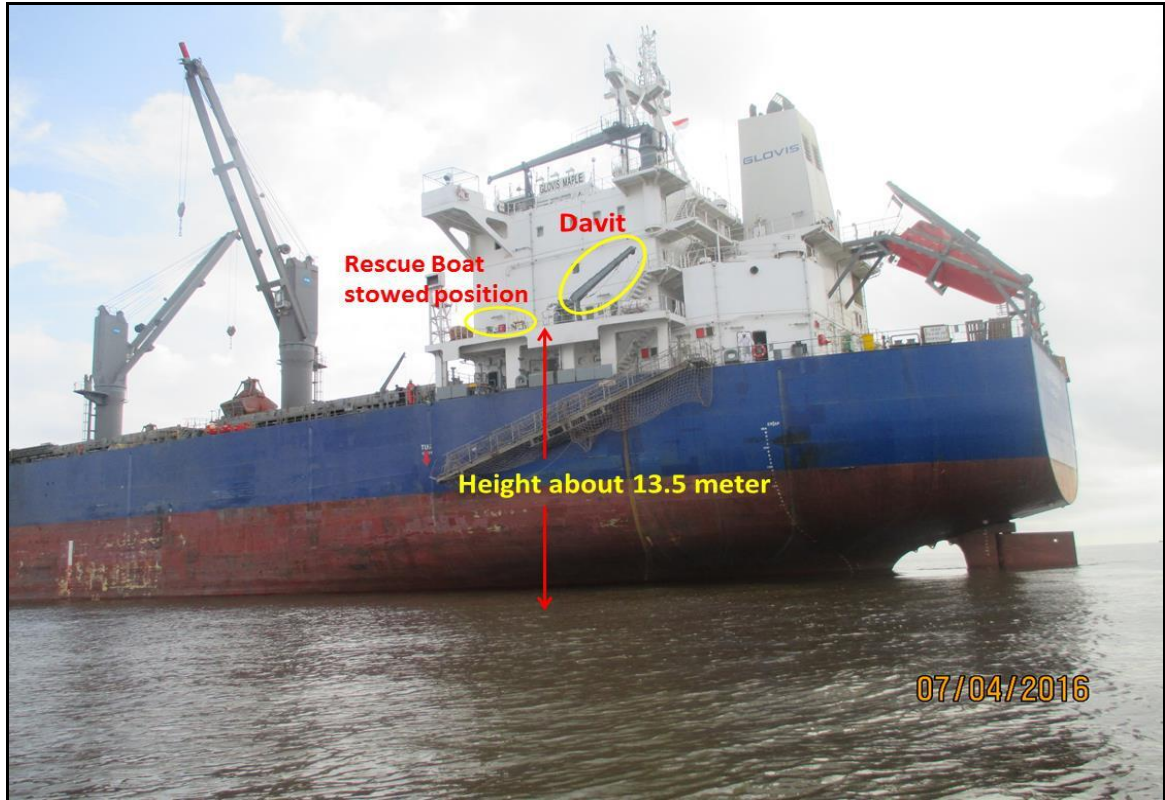
Figure I-8: Rescue boat stowed location
