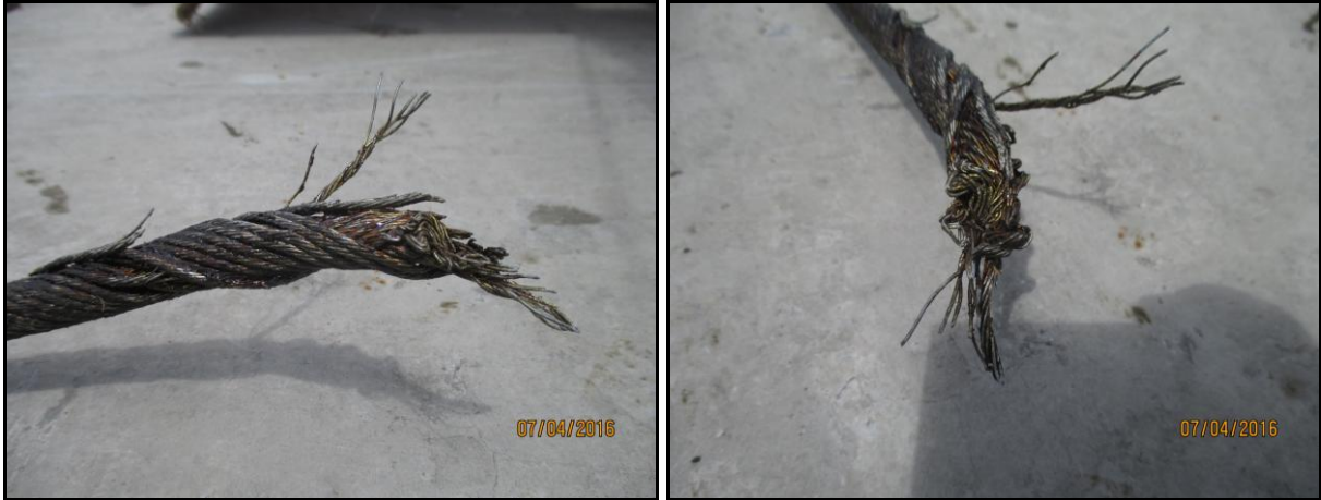
Figure I-15: The failed wire at the hook side (outboard)
