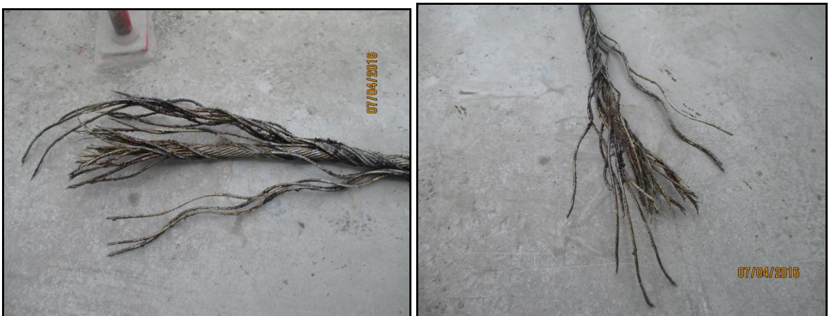
Figure I-16: The failed wire at the winch side (inboard)
