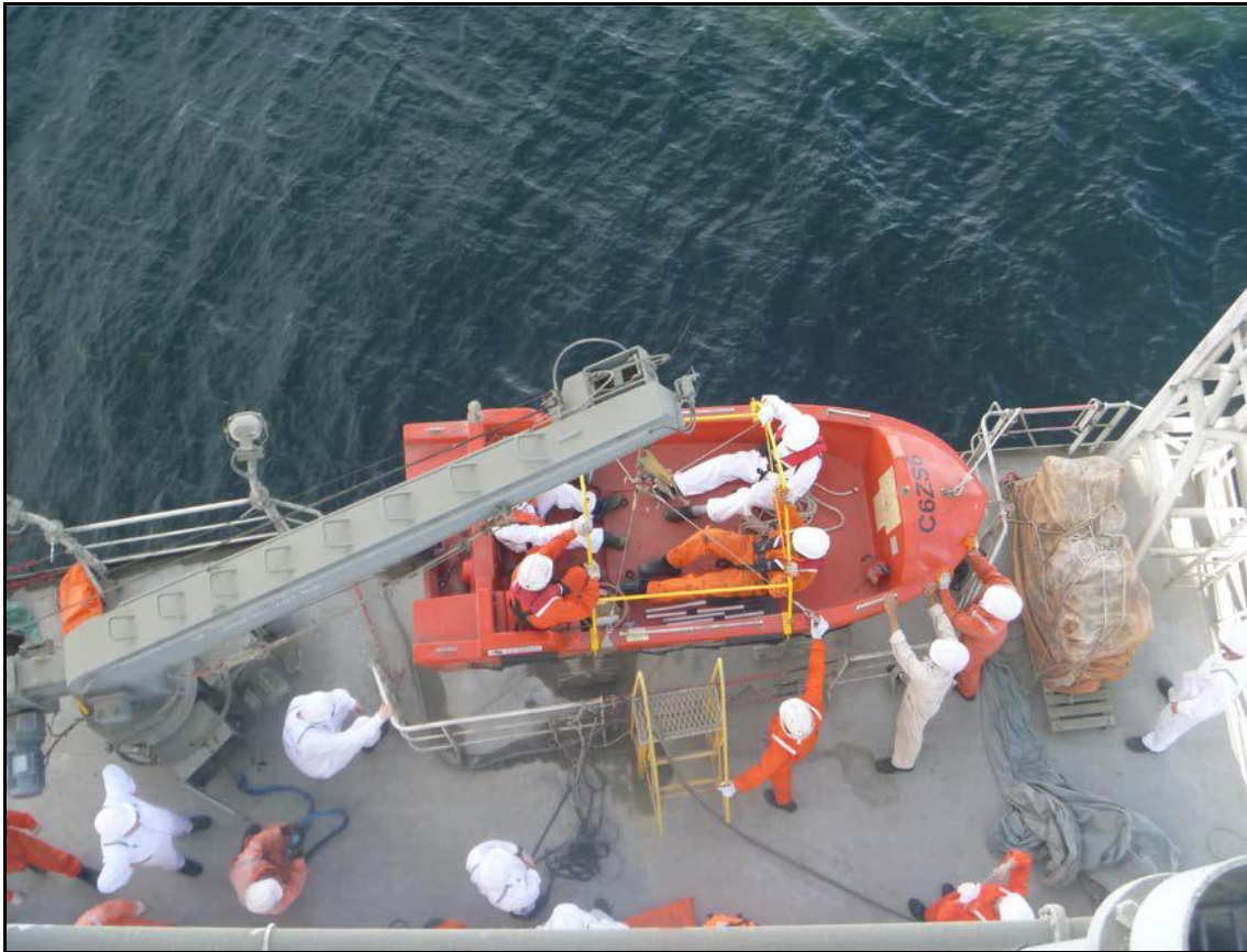
Figure I-7: Crew boarded the boat in stowed position (picture taken by the ship's crew)
