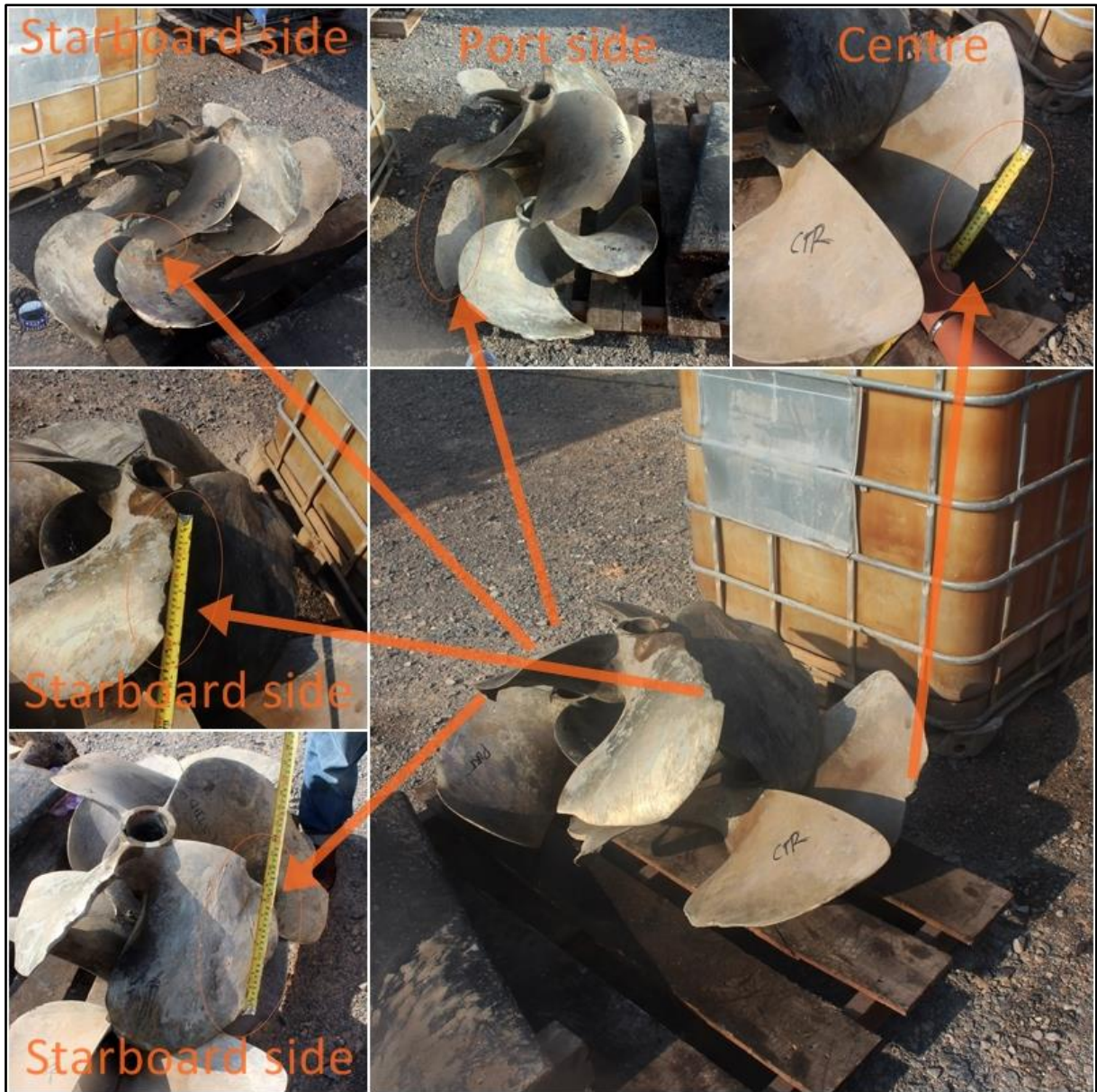
Figure 3: The damages on her propellers
