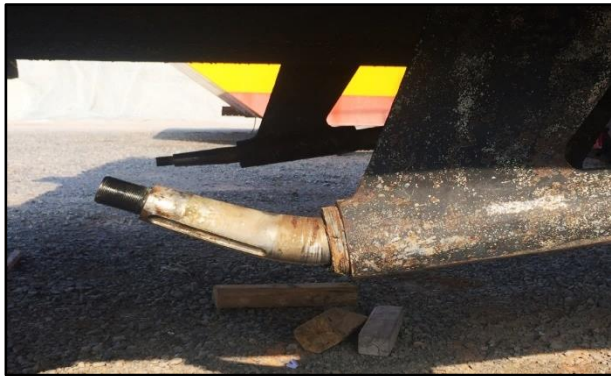
Figure 6: Bended Rudder Post after grounding
