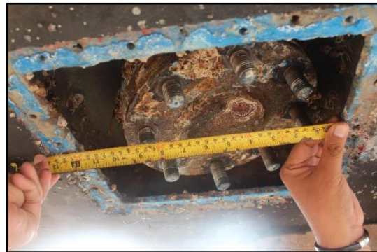
Figure 5: Dented rudder shaft
