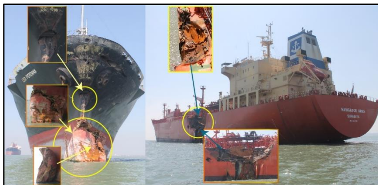
Figure 4: The damaged parts on the LP (left) and NA (right)
