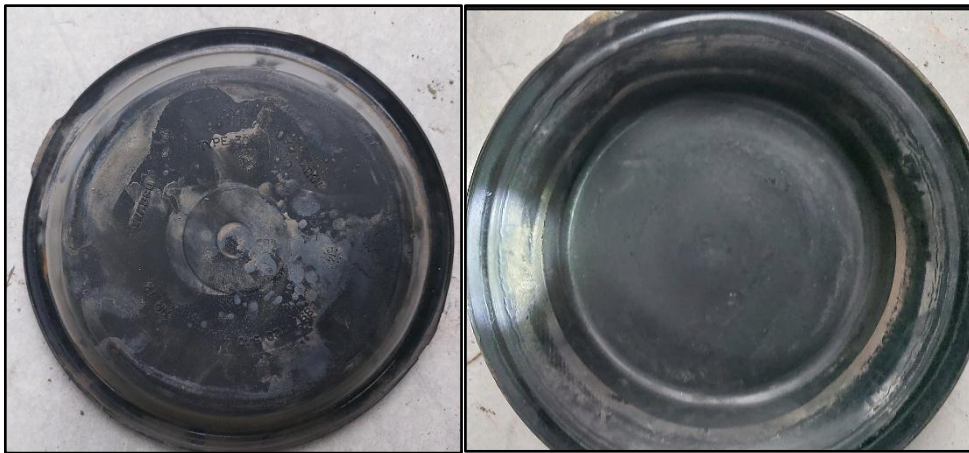
Gambar 25. Diafragma chamber service brake sumbu 3 kanan retak
