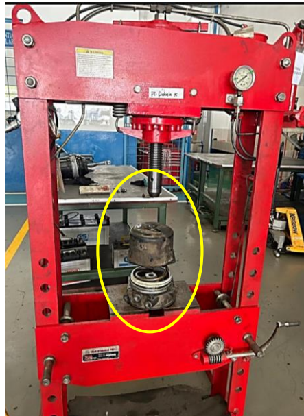
Gambar 24. Proses lepas chamber parking brake
