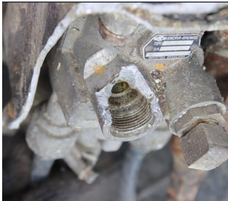
Gambar 8. Brake valve patah akibat tabrakan
