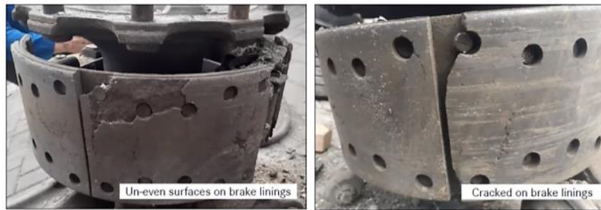
Gambar 30. Ketebalan kampas rem roda kiri 4,7 mm (standar min 7 mm), kondisi pecah
